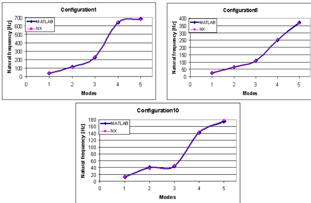
Figure 8: MATLAB and NX5 results comparison
