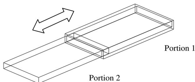
**Figure 3:** Variable length blade (Variblade).
