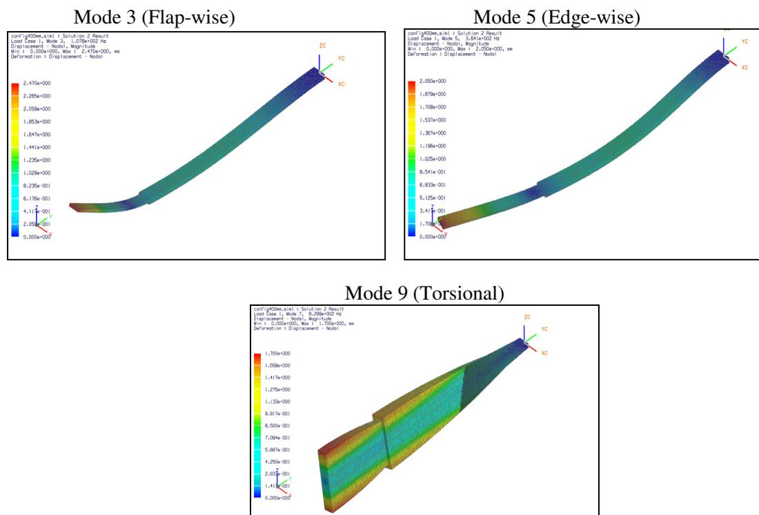
Figure 6: Flap-wise, edge-wise and torsional deflection for configuration 5
