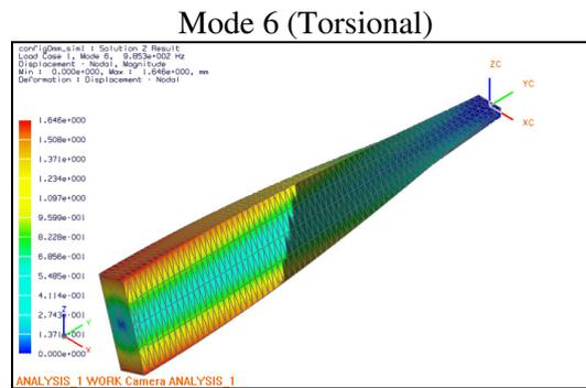
Figure 5: Flap-wise, edge-wise and torsional deflection for configuration 1
