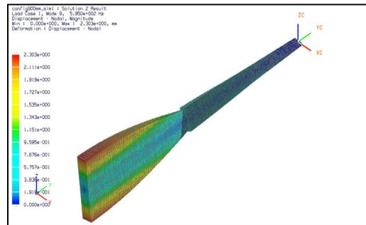
Figure 7: Flap-wise, edge-wise and torsional deflection for configuration 10
