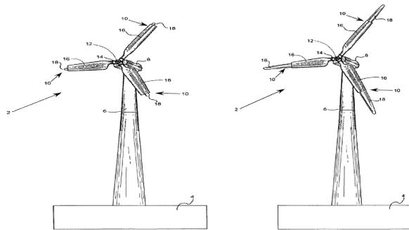
**Figure 1:** Wind turbine with variable length blades with the blades extended and retracted. (Adapted from [2])
