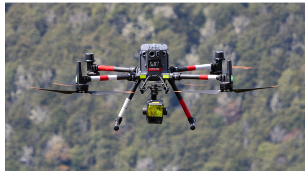
(b) The DJI Matrice 350 UAV-platform equipped with the Zenmuse L2 LiDAR sensor. Image: Copyright by Auckland University of Technology (AUT). Reprinted with permission.
