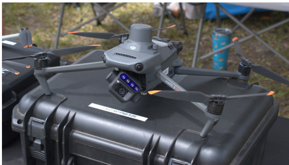
(a) The DJI Mavic 3 Multispectral UAV with the RGB and MS sensors. Image: From wikimedia by ZLEA (2024). CC-BY-SA-4.0.
