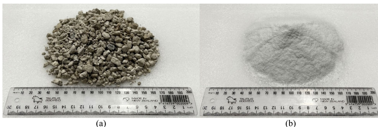
Fig. 1. Images of the (a) coarse pumice sand (PS) and (b) glass powder (GP).
