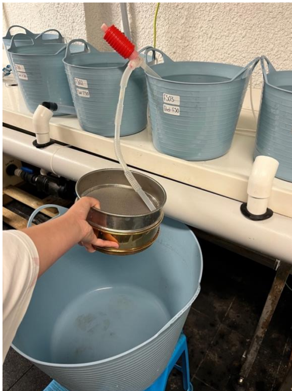
Figure 6: Collection of the uneaten food and faecal matter with a siphon, two sieves, one 150 \mu m sieve and one 80 \mu m sieve and a bucket to collect any unwanted seawater.
