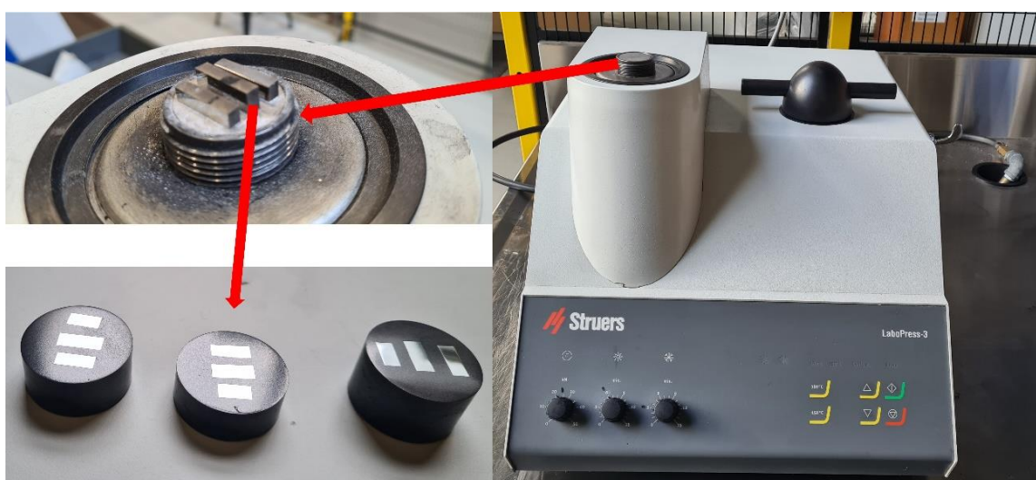
Fig. A.6: Struers hot press mount and the cross-sectional parts of NiTiNOL60 alloy mounted using phenolic resin.
