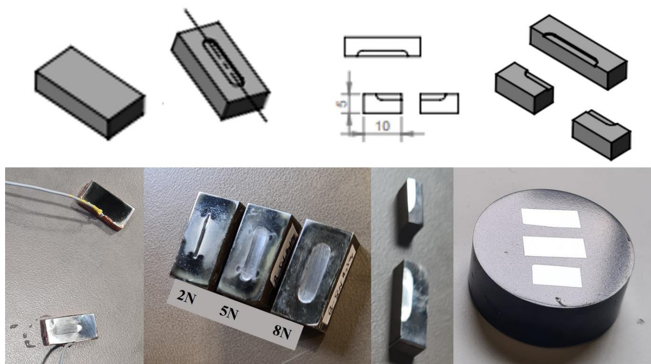
Fig. 9.1: Schematic representation of the sample's geometry and cross-section along the wear track.
