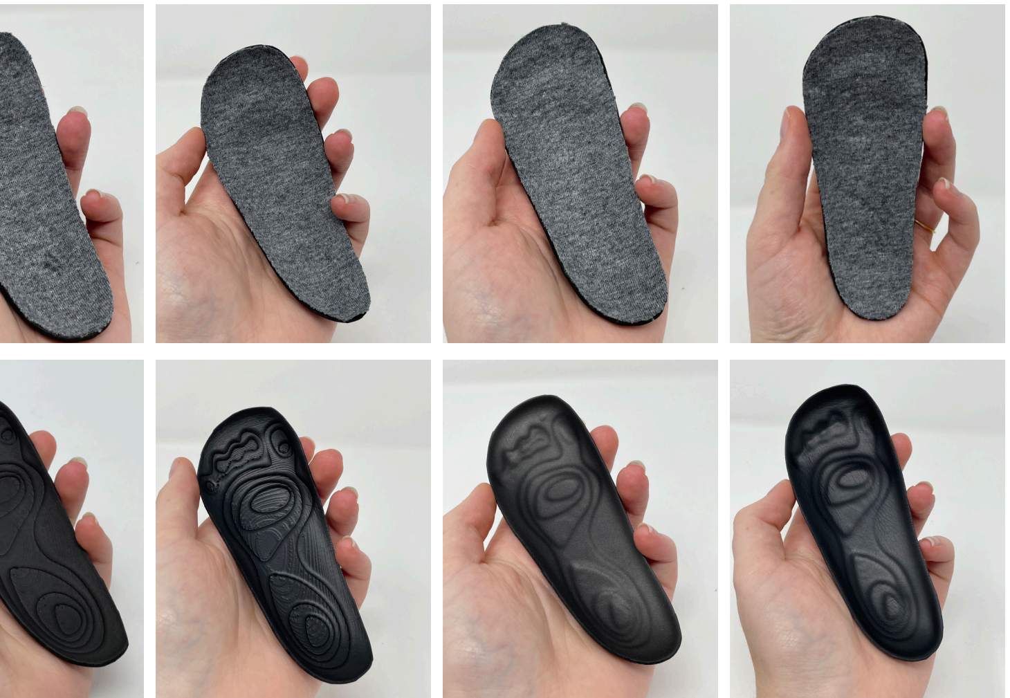
Figure 112. Eight variations of manufacturing techniques for the open-cell foam prototypes, half of the prototypes with cotton glued on, and the other half as only the foam.
