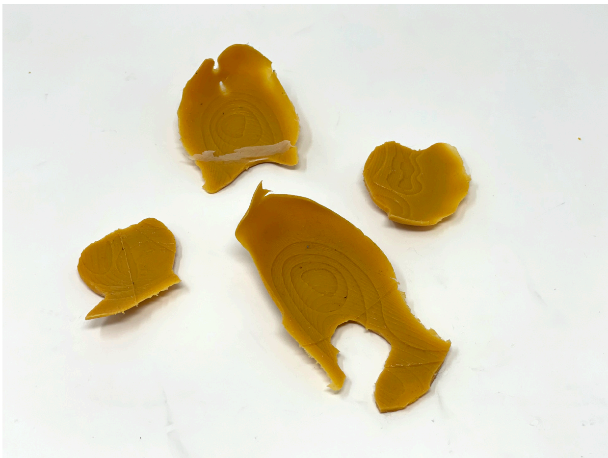
Figure 92. Early attempts at casting the shoe sole which broke apart or did not cure properly.
