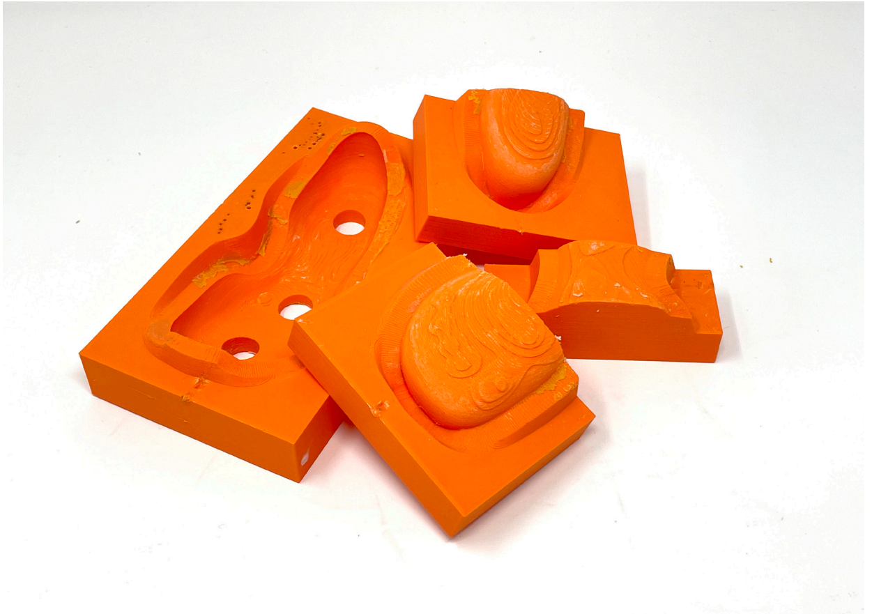
Figure 91. Four part mould of the shoe sole prototype produced for the participant interviews, the mould was used for casting polyurethane.
