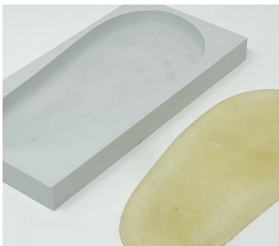
Figure 54. Polyurethane moulds with footprint embedded. Medium imprint depth.
