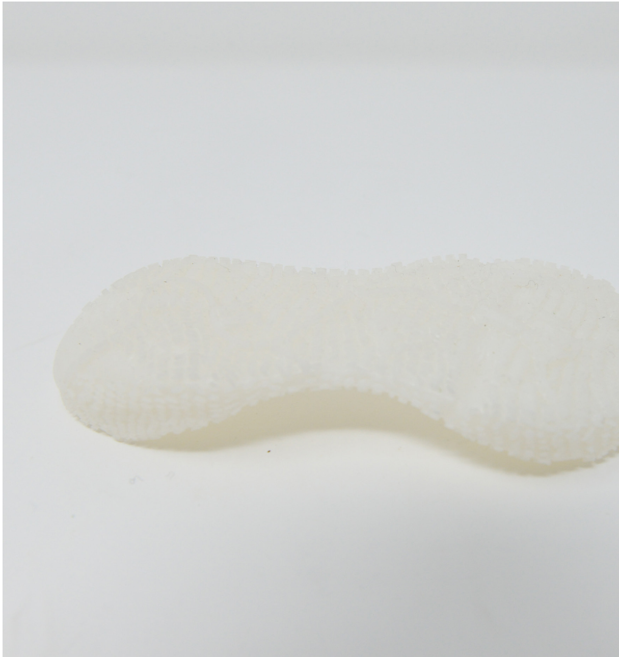
Figure 155. Test print in SLA showing one of the tread patterns with a more pronounced tread depth.
