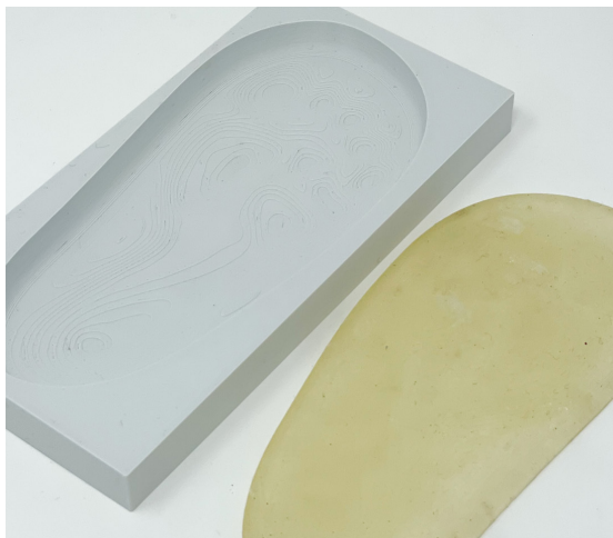
Figure 53. Polyurethane moulds with footprint embedded. Shallow imprint depth.
