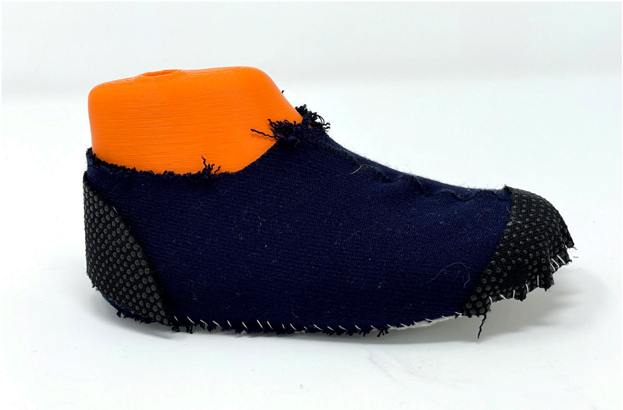
Figure 106. Prototype upper with ceramic dot material on heel and toe cap.
