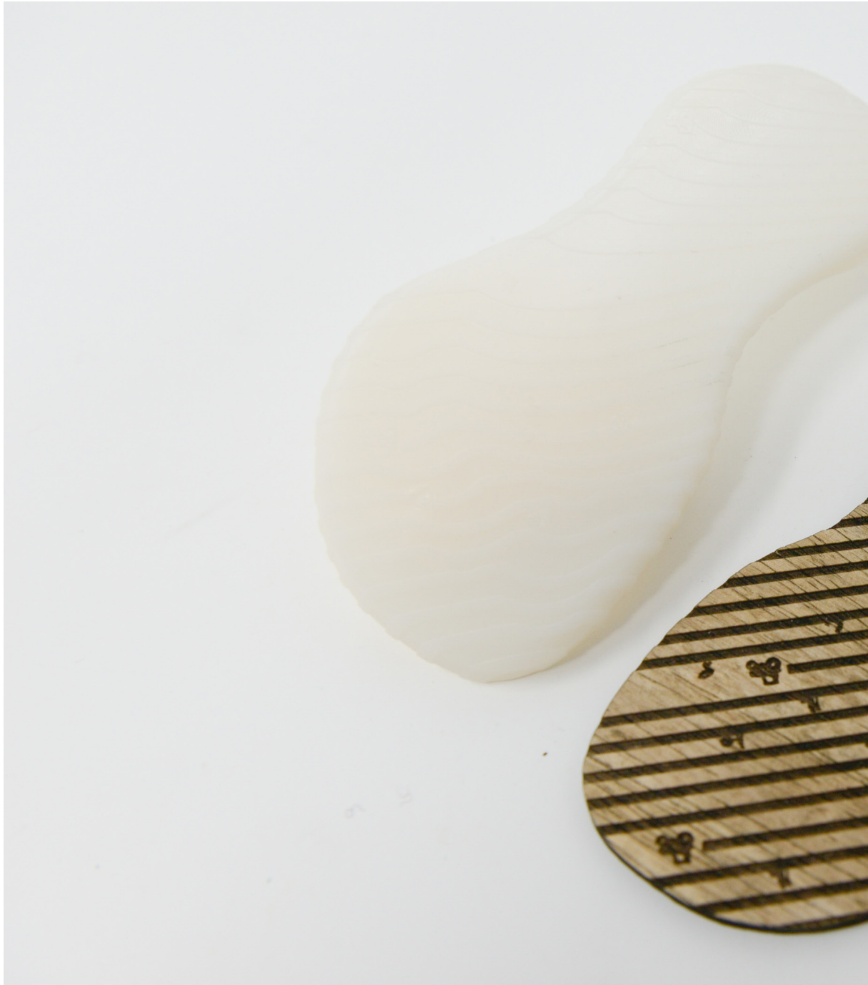
Figure 158. SLA tread print three with laser cut wood pattern demonstrating the print with higher contrast.
