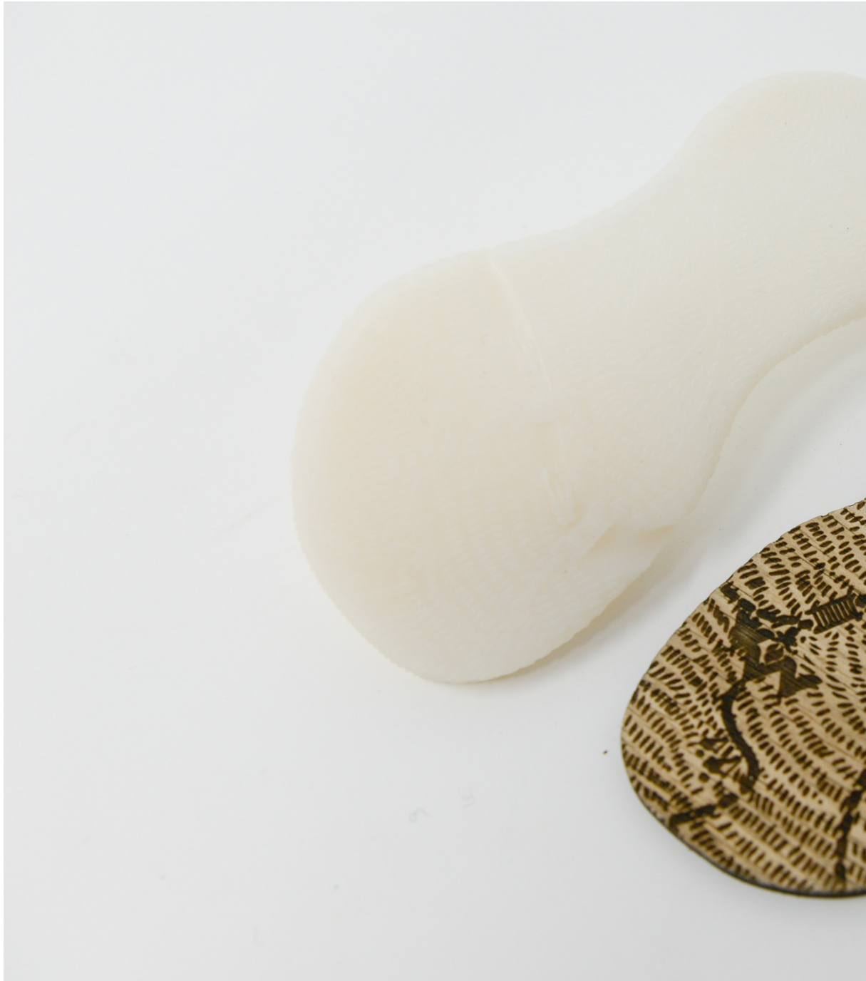
Figure 157. SLA tread print two with laser cut wood pattern demonstrating the print with higher contrast.
