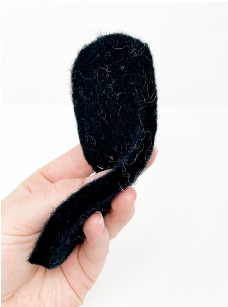
Figure 70. Test insoles using a wool felting loom, testing with various fibres such as regular wool and merino wool.
