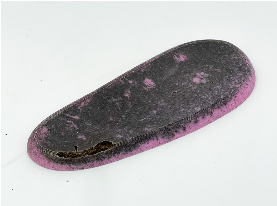
Figure 52. (Top) Prototype using pinkysil silicone, with dirt on the base, aiming to produce a bumpy texture. (Bottom) Prototype using pinkysil silicone, with grass on the base, aiming to produce a grass-like texture
