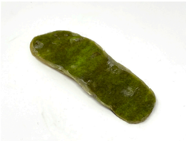
Figure 76. Latex poured over felted wool insole and moulded to a footprint shape to create the imprinted effect with the wool (attached to wool) and latex poured directly over footprint mould to be placed underneath the insole in the shoe (unattached to wool).
