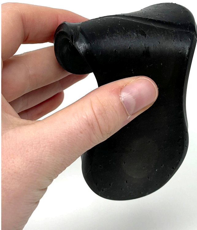
Figure 124. TPU (flexible) 3D printed shoe sole.
