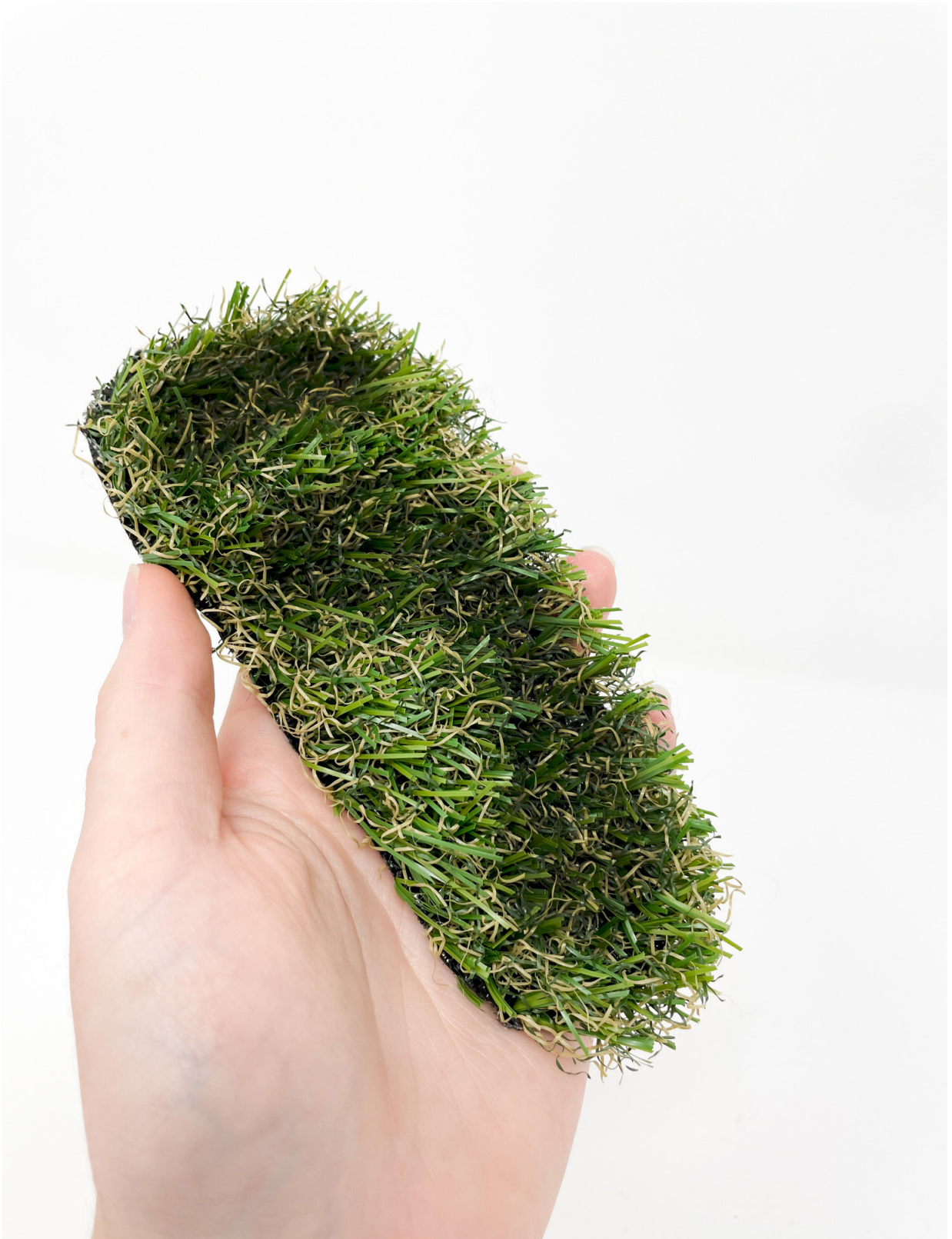
Figure 65. Artificial grass insole cut out with footprint embedded into the grass.
