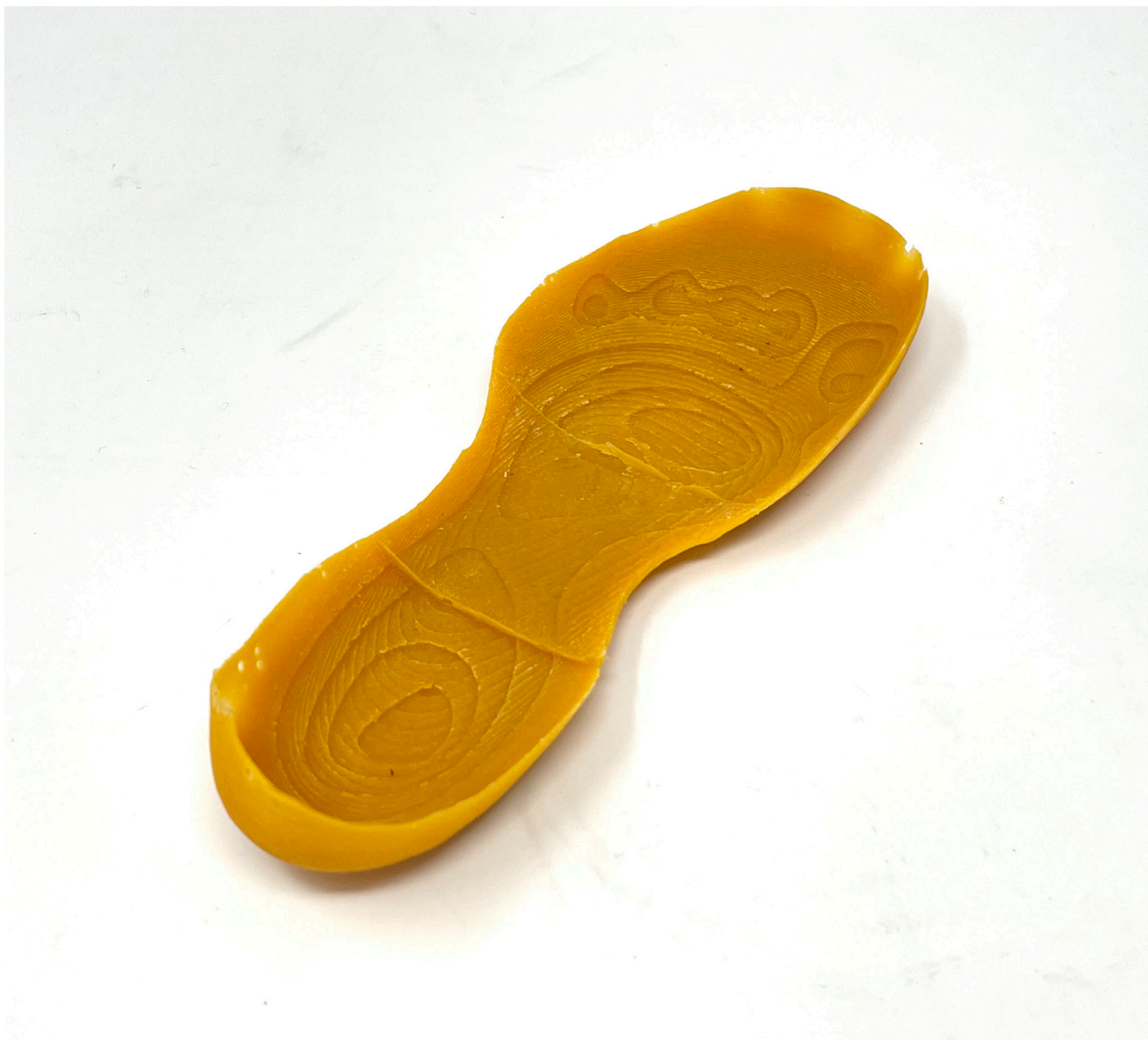
Figure 96. Polyurethane rubber moulded shoe sole sectional model, unattached from the shoe upper because of the time constraints in getting the upper to fit the sole.
