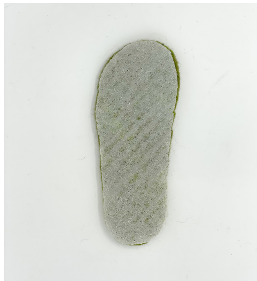
Figure 74. Grassy merino felted onto a piece of woven fabric, cut to insole shape and placed into an existing Bobux sole
