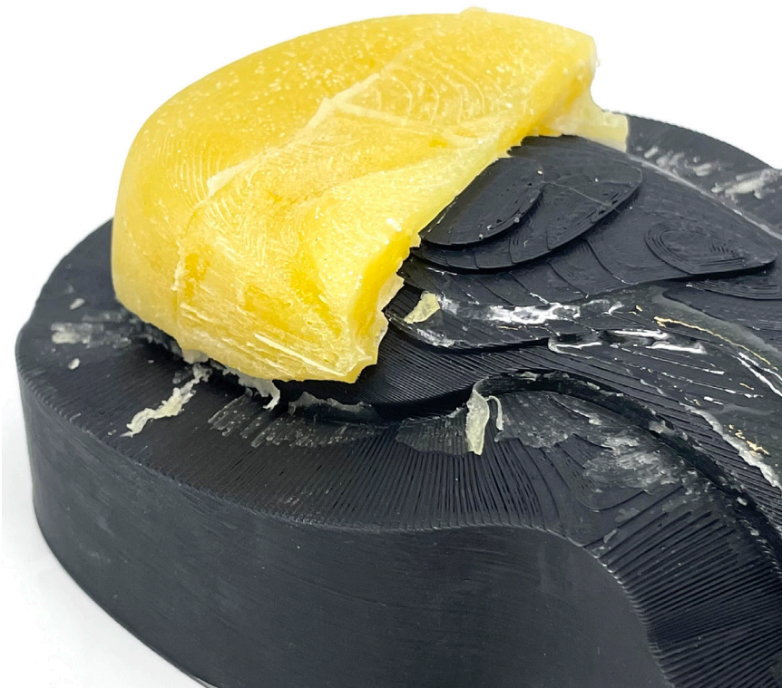
Figure 117. Polyurethane partial mould, showing the contour line on the underside and the thickness of the model which needed to be reduced.
