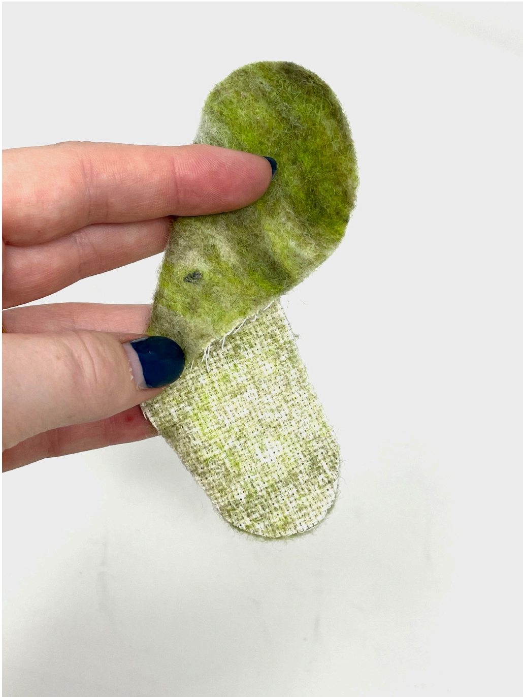
Figure 99. Felted wool sectional prototype sole inner with non-stretch base.
