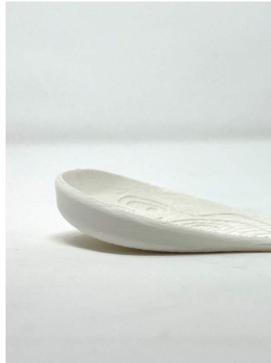
Figure 121. 3D printed shoe sole in solid PLA plastic to ensure the look at the form along with the shoe last.
