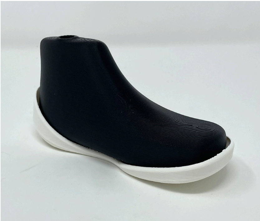
Figure 121. 3D printed shoe sole in solid PLA plastic to ensure the look at the form along with the shoe last.
