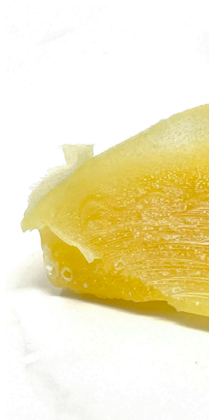
Figure 117. Polyurethane partial mould, showing the contour line on the underside and the thickness of the model which needed to be reduced.
