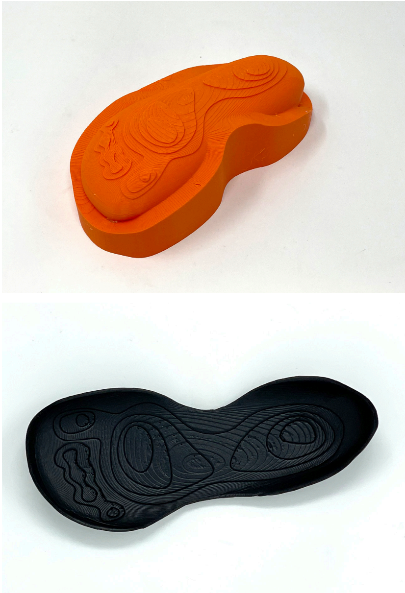
Figure 110. 3D printed vacuum forming mould (Top) and open-cell foam vaccum form shoe footbed (Bottom).
