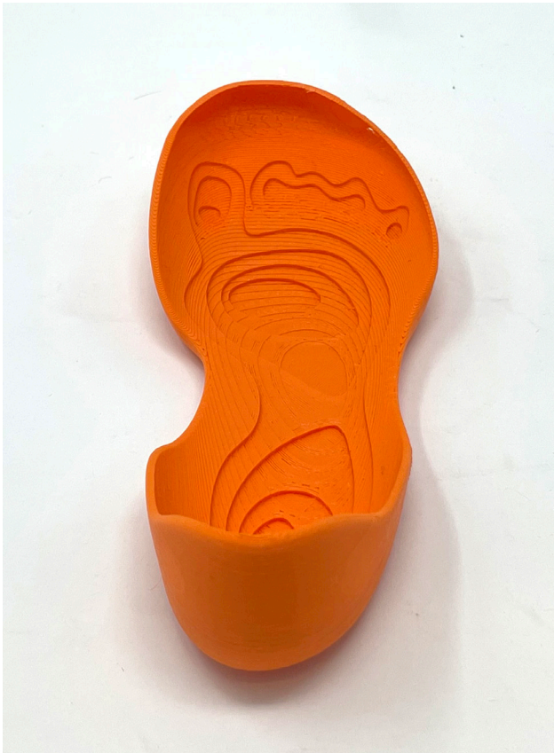
Figure 115. Iteration shows a lighter (less bulky) looking form, with thinner upper edges and a contour line through the toe box on the underside.
