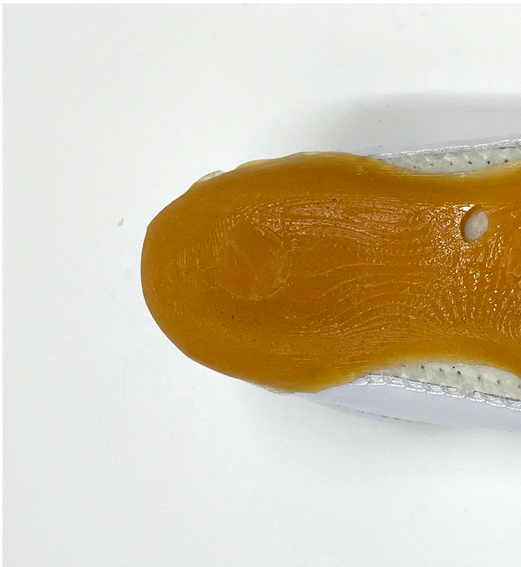
Figure 101. Shoe sole glued onto existing Bobux shoe upper.
