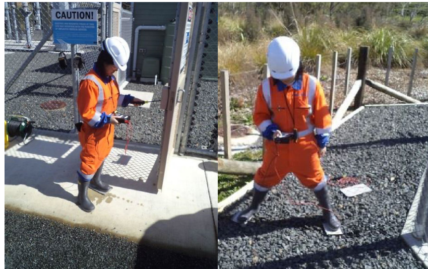
Figure 2-9 Measuring the touch voltage on wet concrete ground (left) and step voltage on crushed rocks (right) in a transmission class substation using the IEEE Std 80 recommended current injection method. The photos were taken by the author in 2014.
