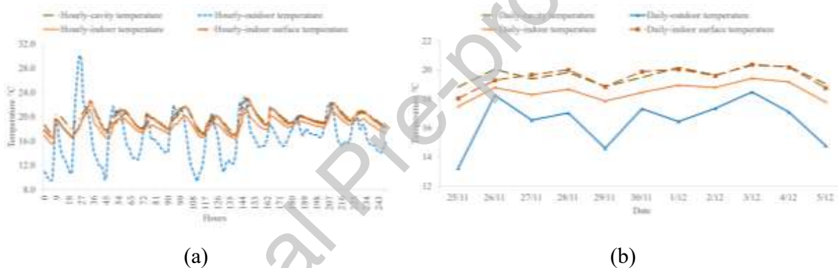
Figure 8 Cavity vs outdoor, surface, and indoor temperature from 25 November until 6 December 2023: (a) hourly and (b) daily.
