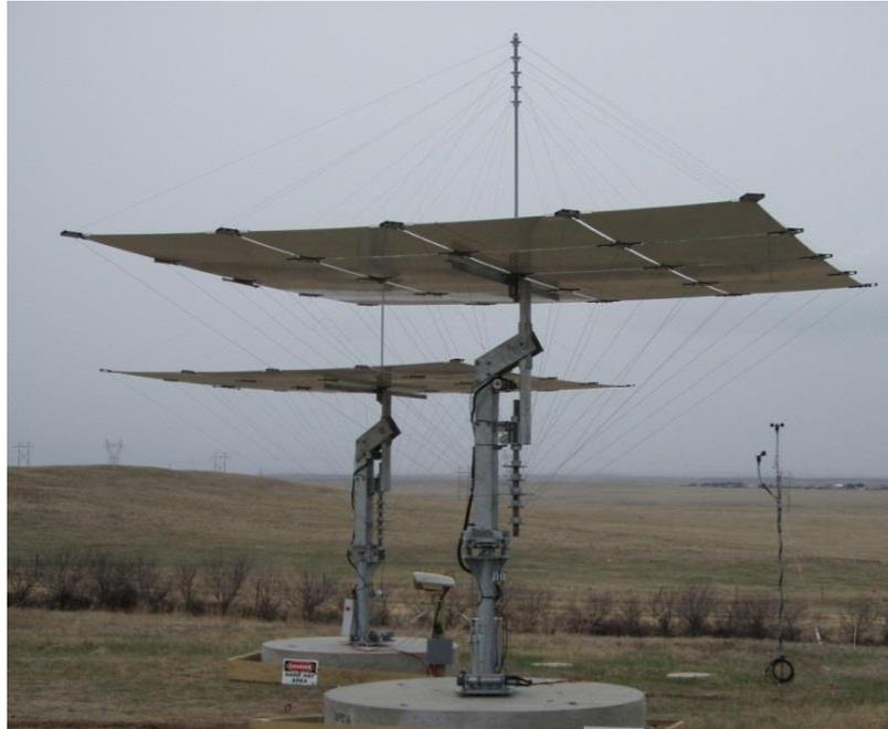
*Figure 15: Solaflect suspension heliostat*
