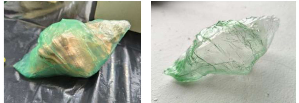
Image 32. (a, b). Testing the casting capabilities of cellulose rice membrane and resulting cuticle cast using a shell, October 2025.
