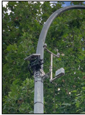
Fig. 10 Example of IoT device that measures weather data, as attached to a nearby streetlight.
