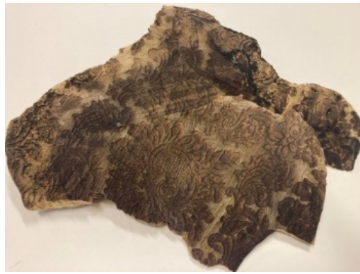
Figures 24, 25 & 26 - Initial concept prototype - ‘Coming together of eras’ – Laser Engraved Flox Damask design onto 115-year-old Macrocarpa. Jay Pressnell 2022. 33 (This specific material experiment had great significance to the eventual proof of concept outcomes, as it firstly brought together two emotive materials, one a slice of timber that came off a 115 year old tree on my land, the other a significant wallpaper design which adorned the walls of my grandparents house in South London. Bringing them together felt like a powerful union of generations, whilst the material fusion felt complementary and cohesive).
