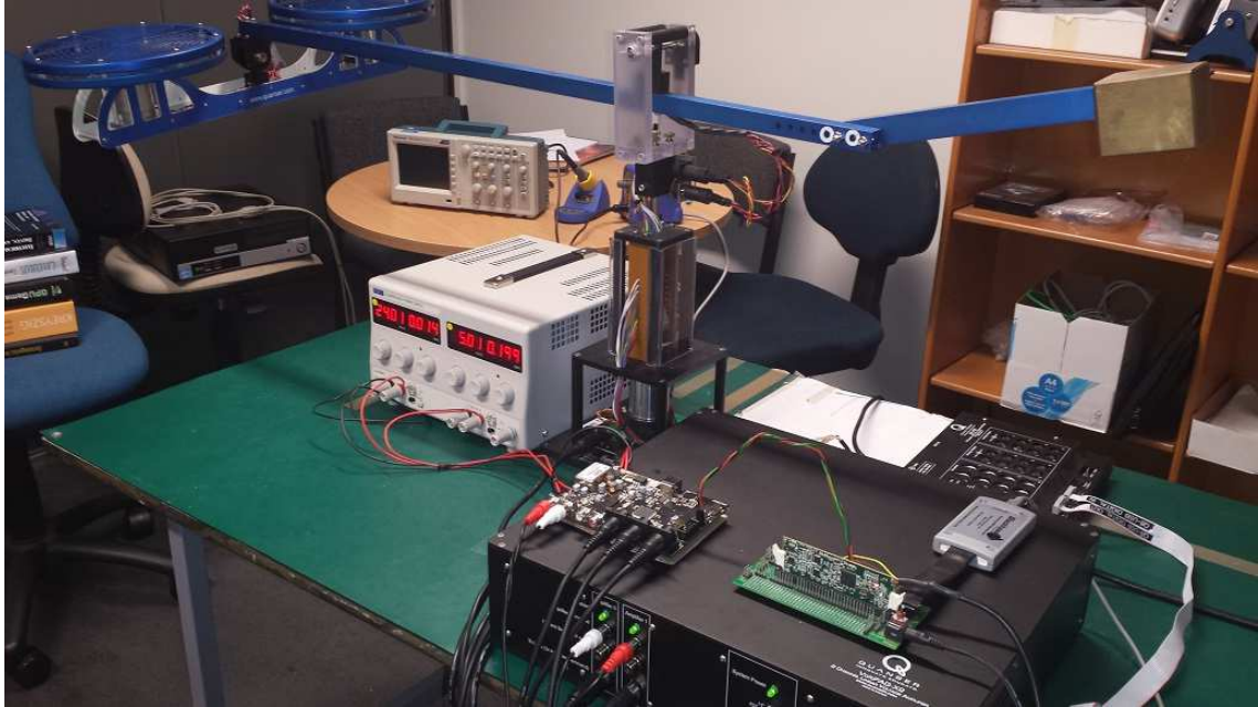
Figure 4.29: 3DOF Helicopter complete hardware setup including the TI C28343, custom DAQ, Quanser amplifier, benchtop powersupply and 3DOF helicopter.
