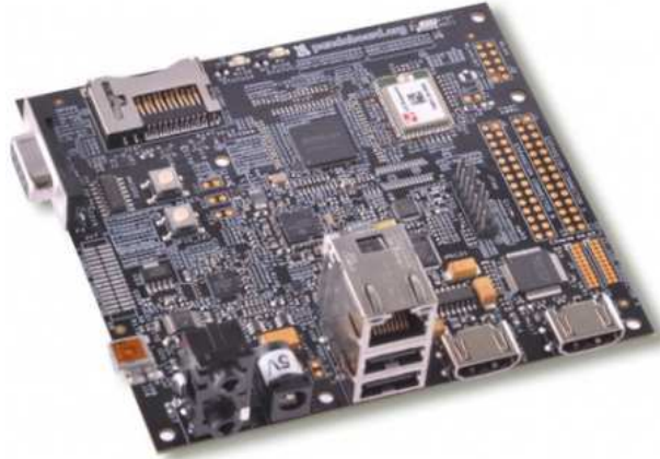
Figure 4.2: PandaBoard with dual core ARM Cortex A9 [344].
