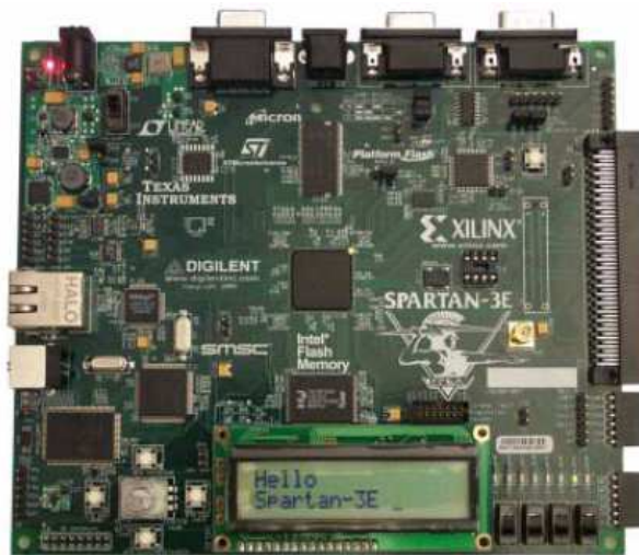
Figure 4.4: Xilinx Spartan 3E starter board [341].
