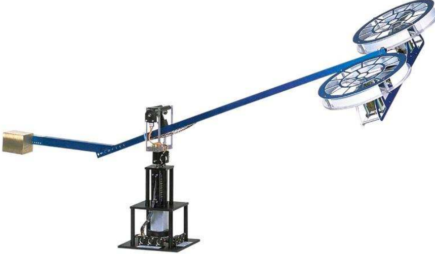
Figure 4.24: Quanser 3DOF Helicopter plant [268].
