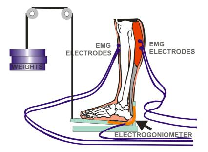
Figure 1. A schematic representation of the apparatus used to measure dorsiflexion range of motion of the ankle.
