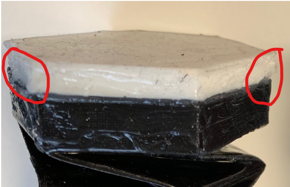
(a) Air leakage in design 1
