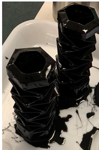
Figure 4.6: Fabricating origami cylinder by sinking in silicone
