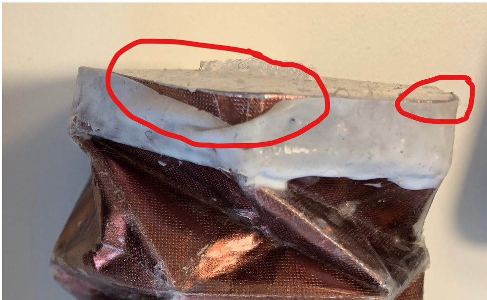
(b) Air leakage in design 2
