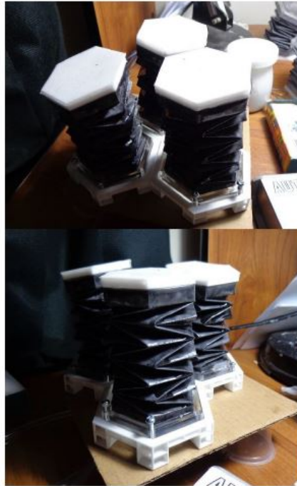
Figure 2.5: First prototype of the origami table robot (Maratas, 2018)
