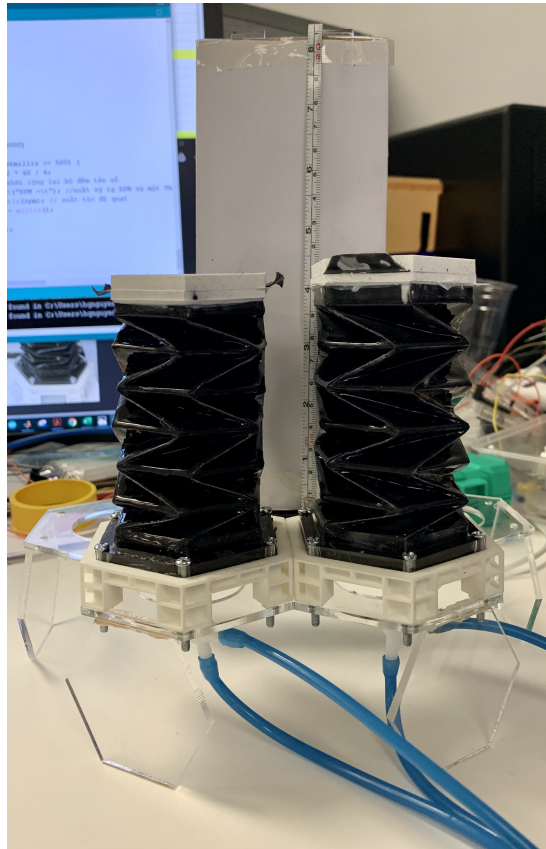
Figure 5.9: Measuring configuration with two actuators
