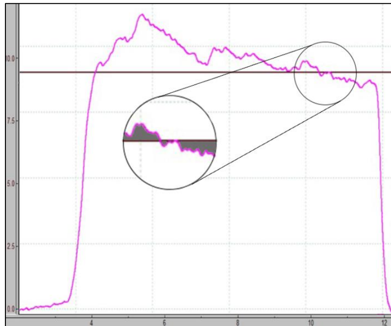
Figure 5. Visual representation of torque matching accuracy (RMS). The shaded area represents the difference between the participant's produced torque (magenta line) and the target torque (black line).
