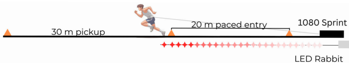
Figure 1. Sprint lane setup for pickup acceleration testing showing distances and locations of technology used.
