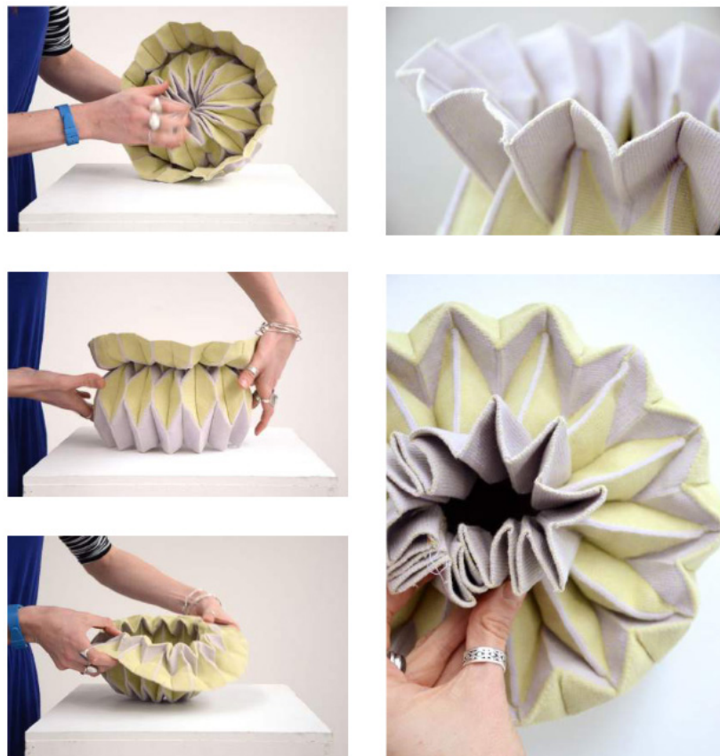
Figure 38. Digitally knitted origami inspired forms using cotton and thermoplastic yarns to create form by Victoria Salmon. Reproduced from Victoria Salmon, "Dynamic Folding Knits: Play // Interact // Explore" (master's thesis, University of Borås, 2020), 69, https://www.diva-portal.org/smash/get/diva2:1455073/FULLTEXT01.pdf .
