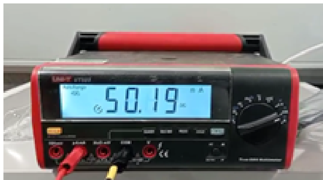
Figure 8.3: . Max current reading from ground test is 50.19mA.
