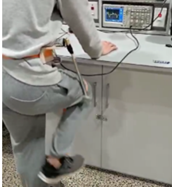
Figure 8.2: Ground test in AUT lab. The participant is leaning to one side to ensure the floor does not impede the leg's free motion.
