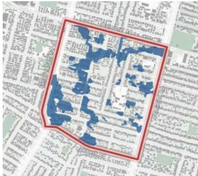
Figure 101: Flood prone areas within site
