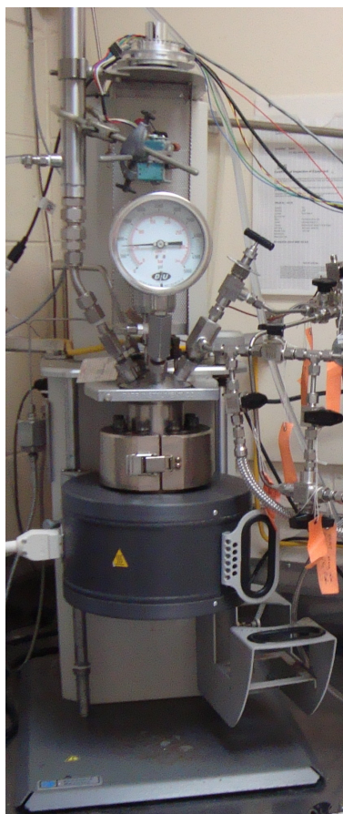
Figure 3.7: Parr reactor with the replacement stirrer motor fitted.
