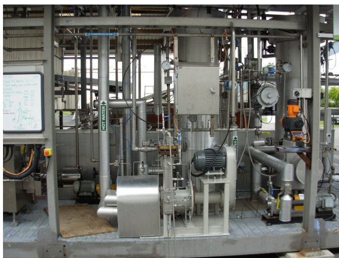
Figure 3.10: The main bubble column reactor with the liquid recirculation pump in the foreground.
