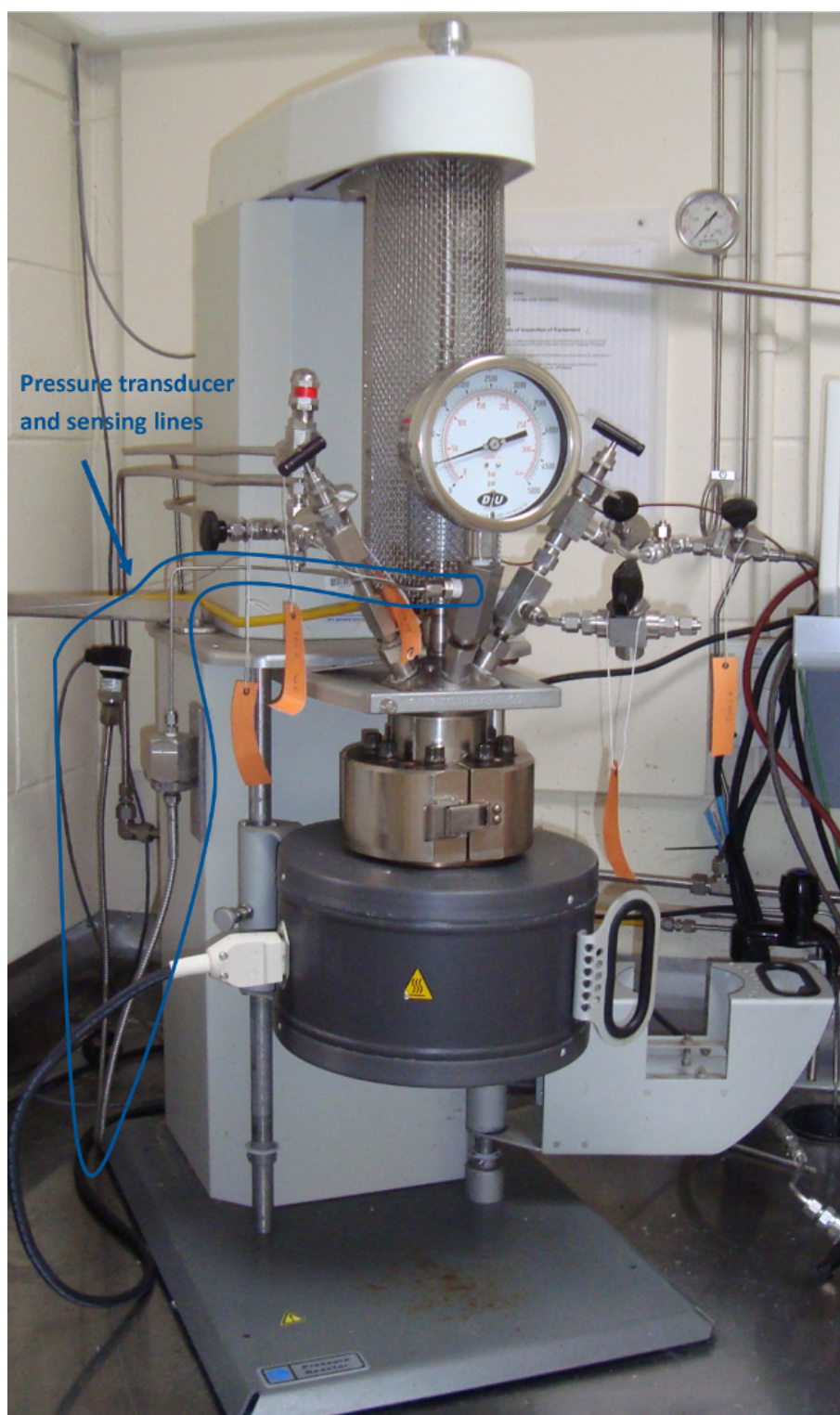
Figure 5.30: Lab scale Parr reactor with the pressure measurement system highlighted.
