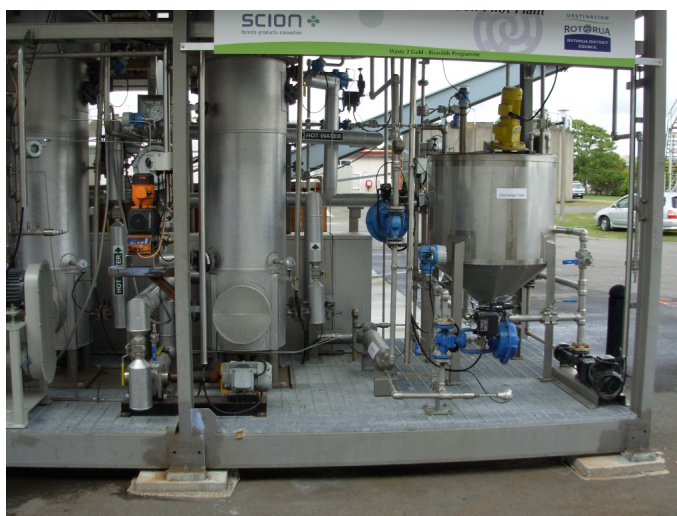
Figure 3.11: The secondary bubble column reactor and discharge tank.
