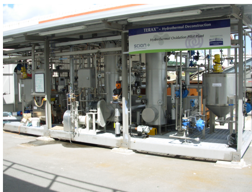
(b) TERAX stage 2: Wet oxidation unit with two 300L reactors
