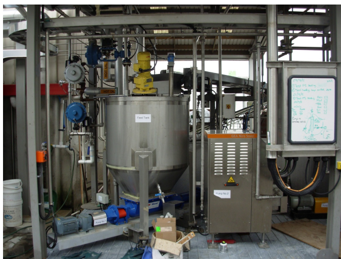
Figure 3.9: The TERAX wet oxidation pilot plant feed tank and high pressure feed pump. The feed pump is to the right of the feed tank.
