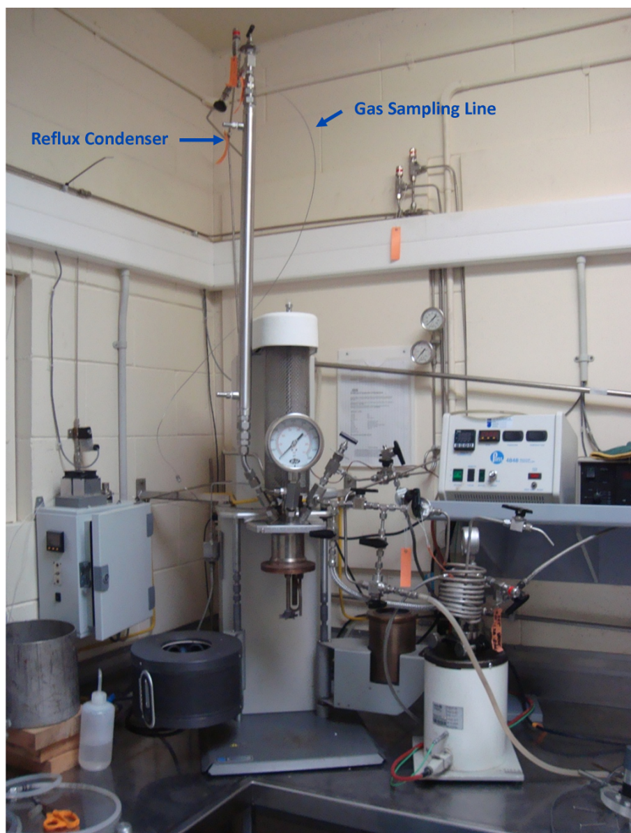
Figure 5.20: Photograph showing the reflux condenser installed on the gas outlet of the Parr reactor and the location of the off-gas sampling line.
