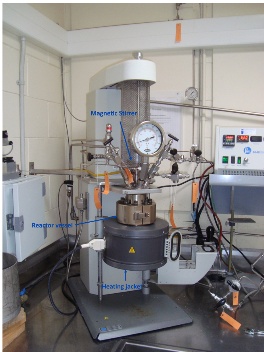
Figure 3.2: The 4540 Parr reactor and 4848 controller (schematic shown in Fig. 3.1).
