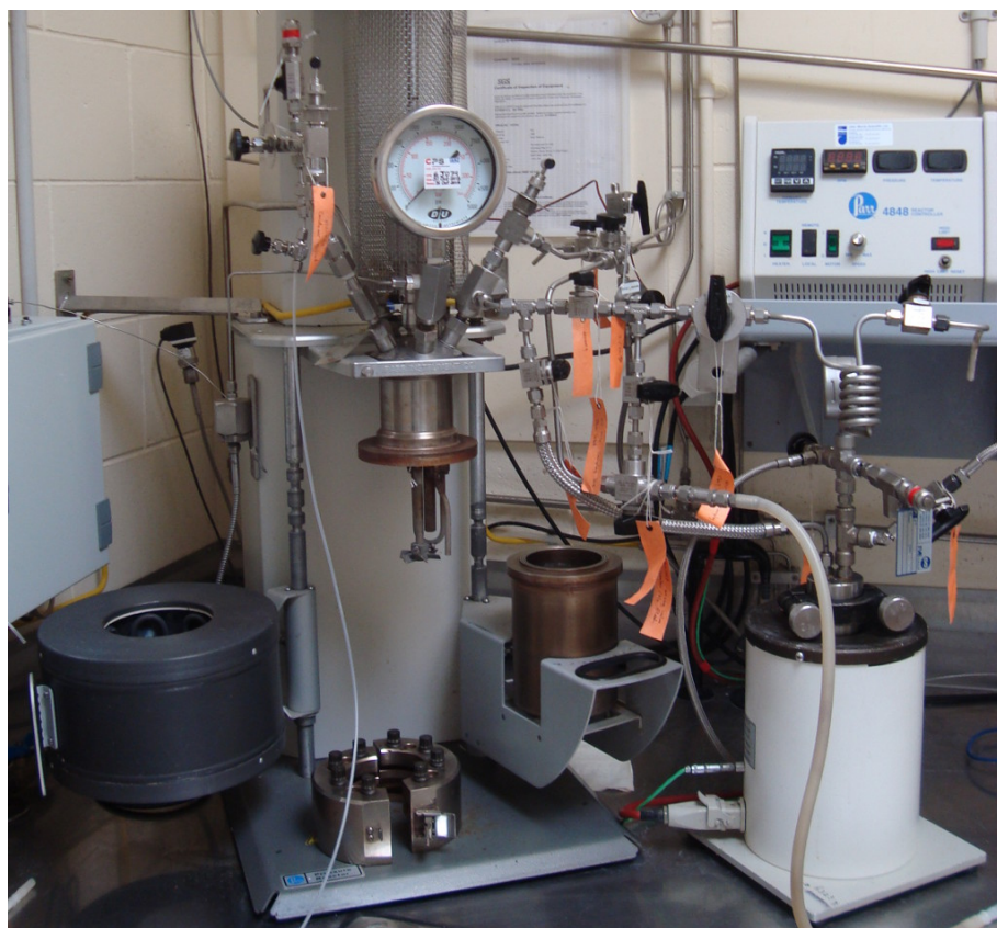
Figure 3.5: The Parr reactor with the added sampling and injection system.
