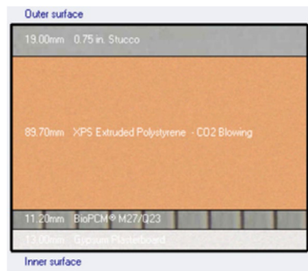
Fig. 2. BioPCM Q23 based building envelop system.
