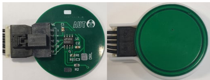
Figure 2-4: active capacitive electrode
