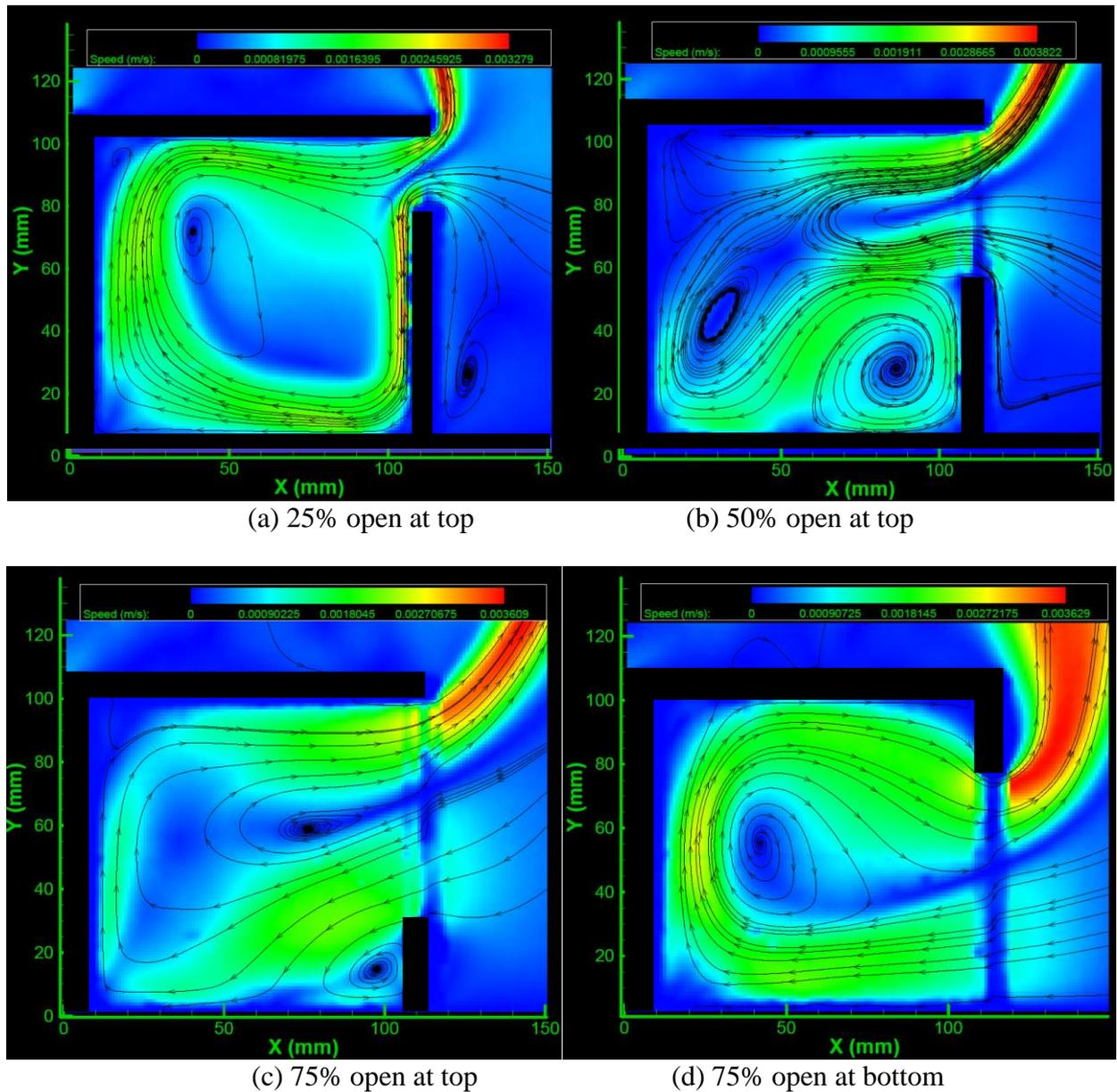
Fig. 5 Streamlines and velocity contours for enclosures at  $200\text{W}/\text{m}^2$
