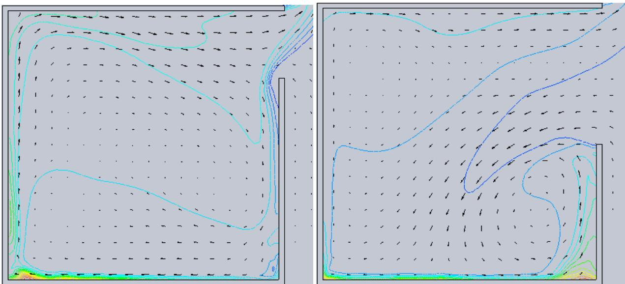
Fig. 3 Flow in an open enclosure with various opening sizes (25% left, 50% right)
