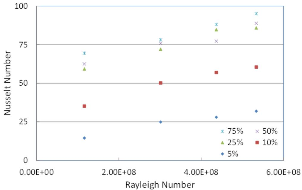
Fig. 2 Nusselt v Rayleigh Number for an open enclosure with various opening sizes
