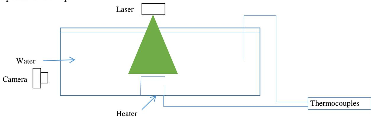
Fig. 4 Schematic of experimental apparatus
