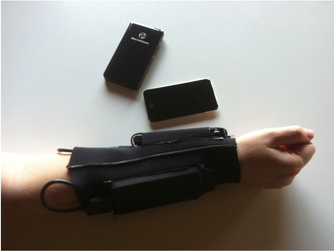
Figure 4. A pico projector, an iPod Touch and neoprene sleeve turn S.A.R.A. into a wearable dance device.
