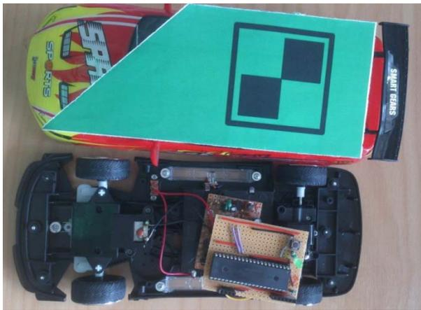
**Figure 4 Modified RC vehicle with polygon and pattern**
