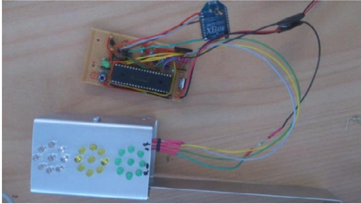
**Figure 5 Traffic Signal (Showing Internals)**
