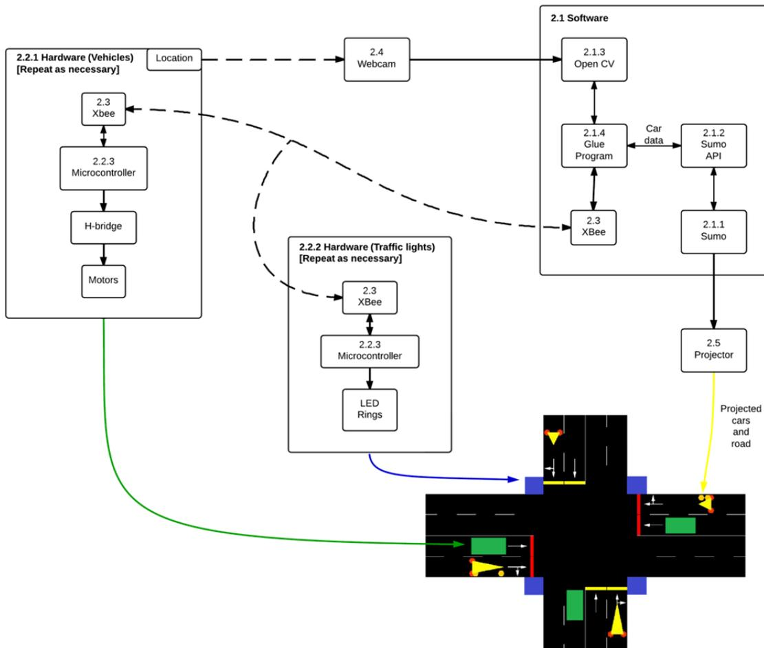
Figure 1: ITS Demo Environment System Diagram and Physical Setup
