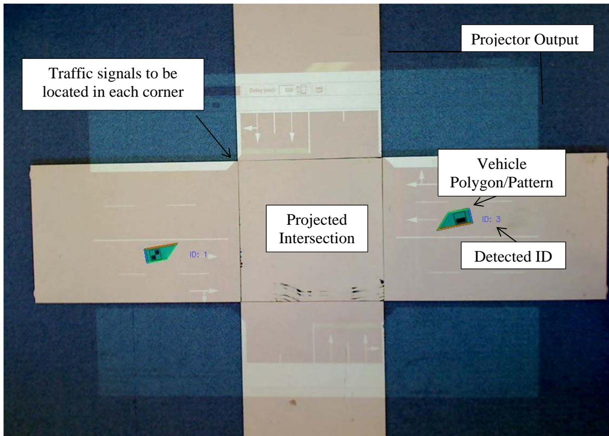
**Figure 3 OpenCV Image Processing of the ARDE**
