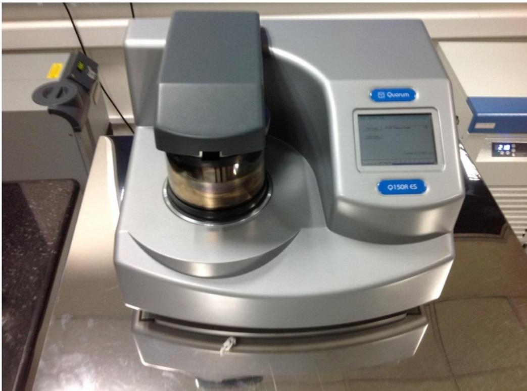
**Figure 4-7: Q150R Rotary-Pumped Sputter Coater/SEM Carbon Coater.**
