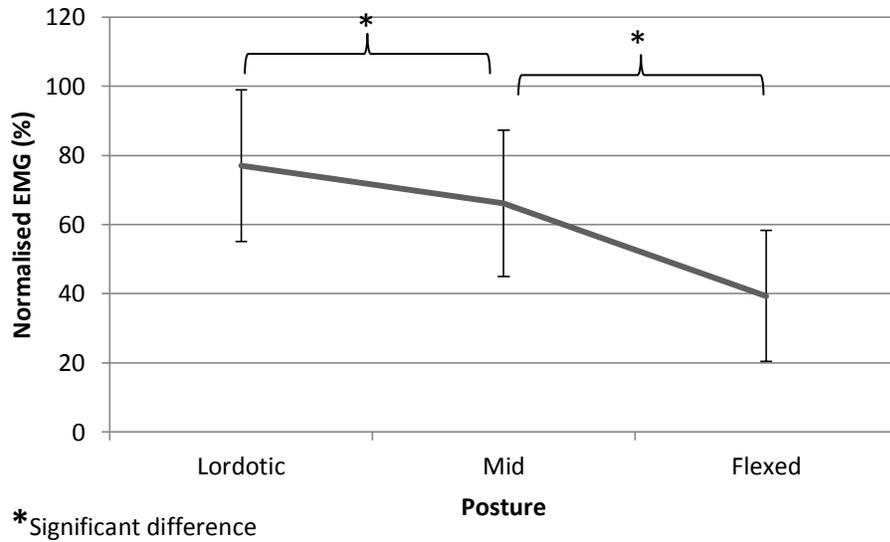
**Figure 4.7** Normalised EMG for each lifting posture
