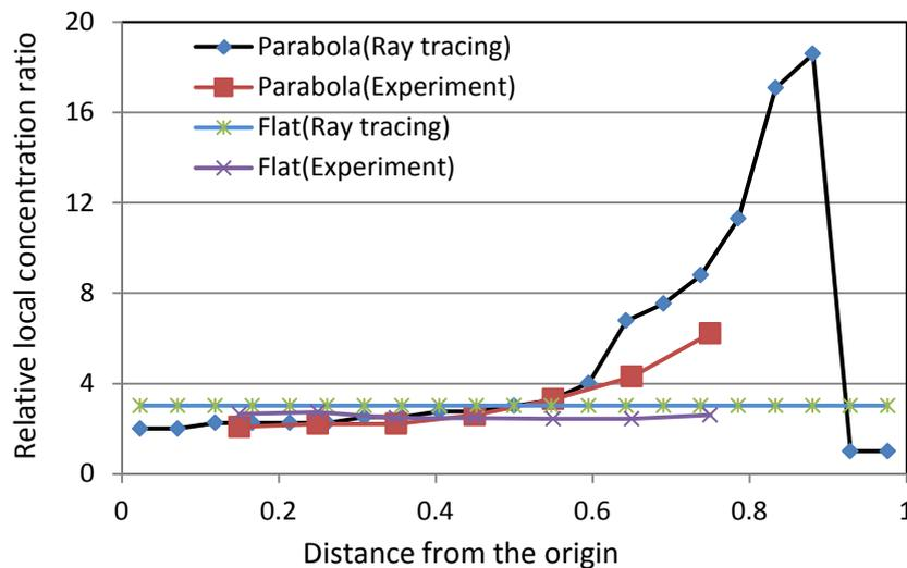
Figure 8 Relative local concentration ratios across the absorber at 30 degree elevation angle
