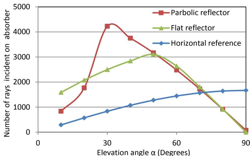
Figure 2 Number of rays hitting the absorber v elevation angle ( $\alpha$ ) of the source
