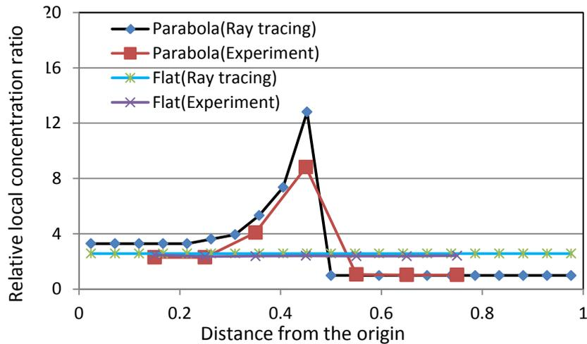
Figure 9 Relative local concentration ratios across the absorber at 45 degree elevation angle
