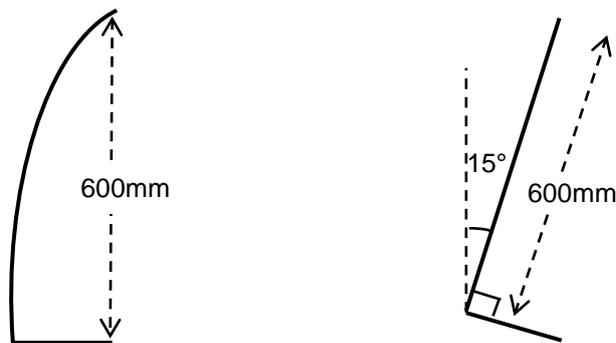
Figure 6. Schematic diagrams of the reflectors
