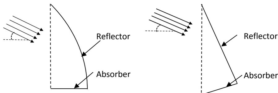
Figure 1 Façade integrated concentrator profiles
