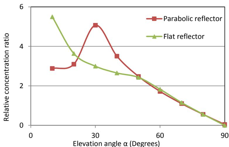
Figure 3 Elevation angle v relative concentration ratio
