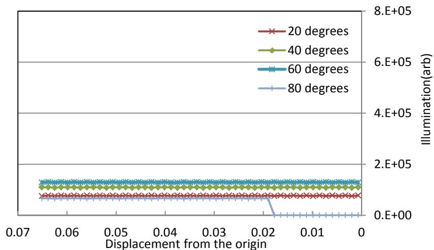
Figure 5 Illumination on the absorber module at various elevation angles under flat reflector
