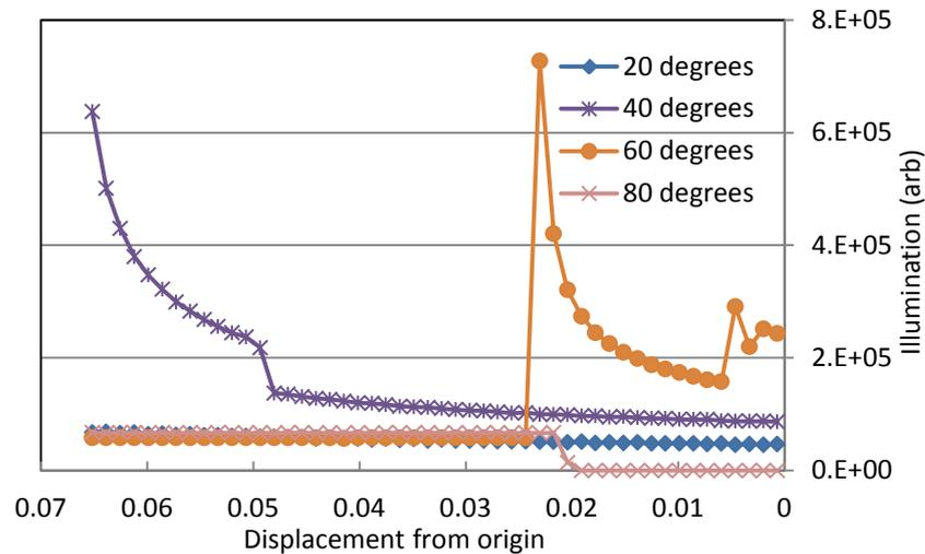
Figure 4 Illumination on the absorber module at various elevation angles under parabolic reflector
