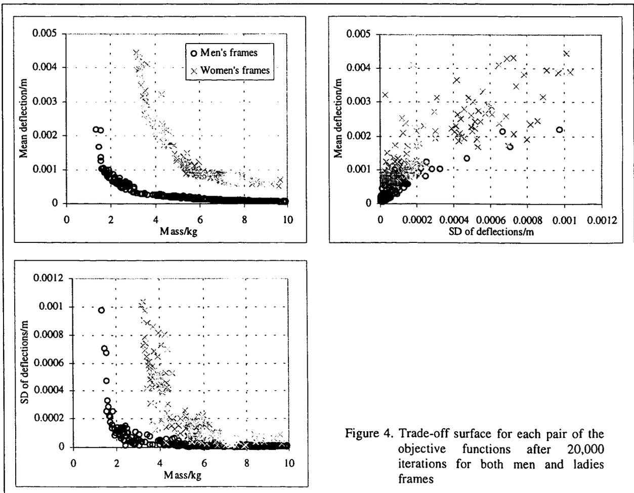
Figure 4. Trade-off surface for each pair of the objective functions after 20,000 iterations for both men and ladies frames
