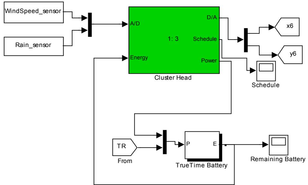
Figure 8.9: The Micro-scale FWI system cluster head sub-model.
