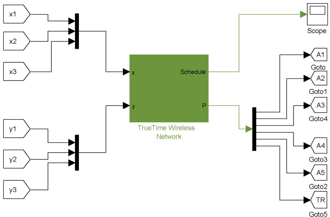
Figure 6.7: The TrueTime Wireless Network Model.
