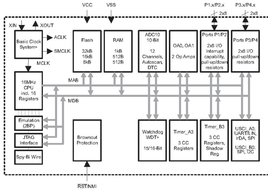
Figure 3.8: MSP430F2274 Functional Block Diagram.
