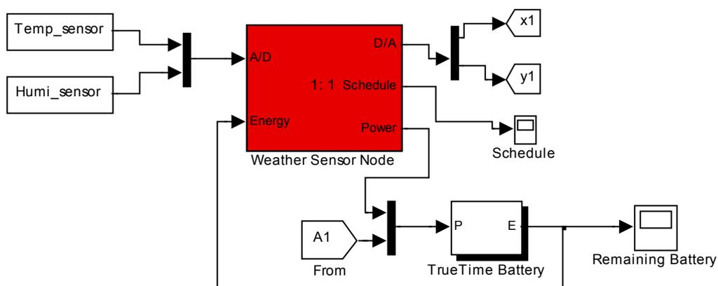
Figure 8.8: The Micro-scale FWI system weather sensor node sub-model.
