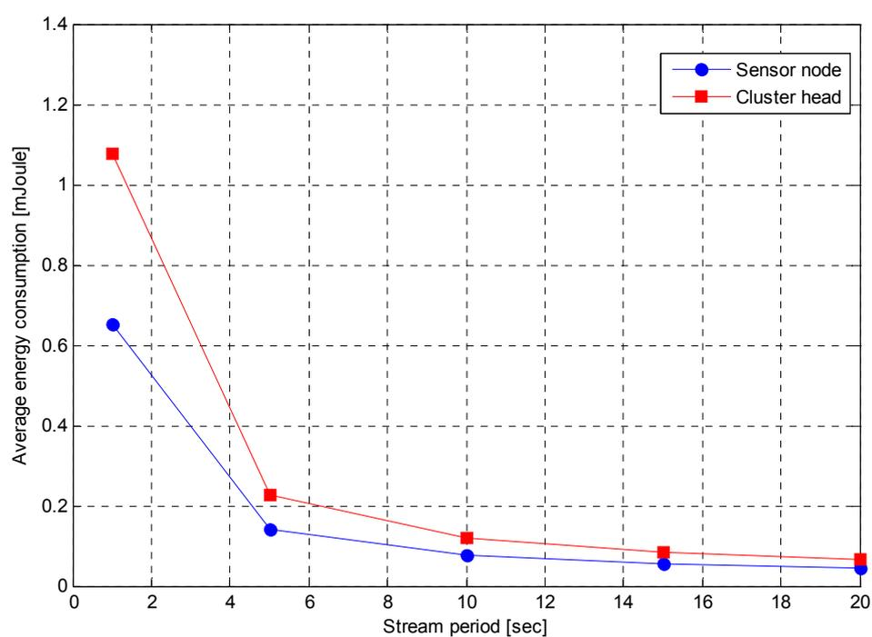
Figure 7.22: Sensor nodes and cluster heads average energy consumption.
