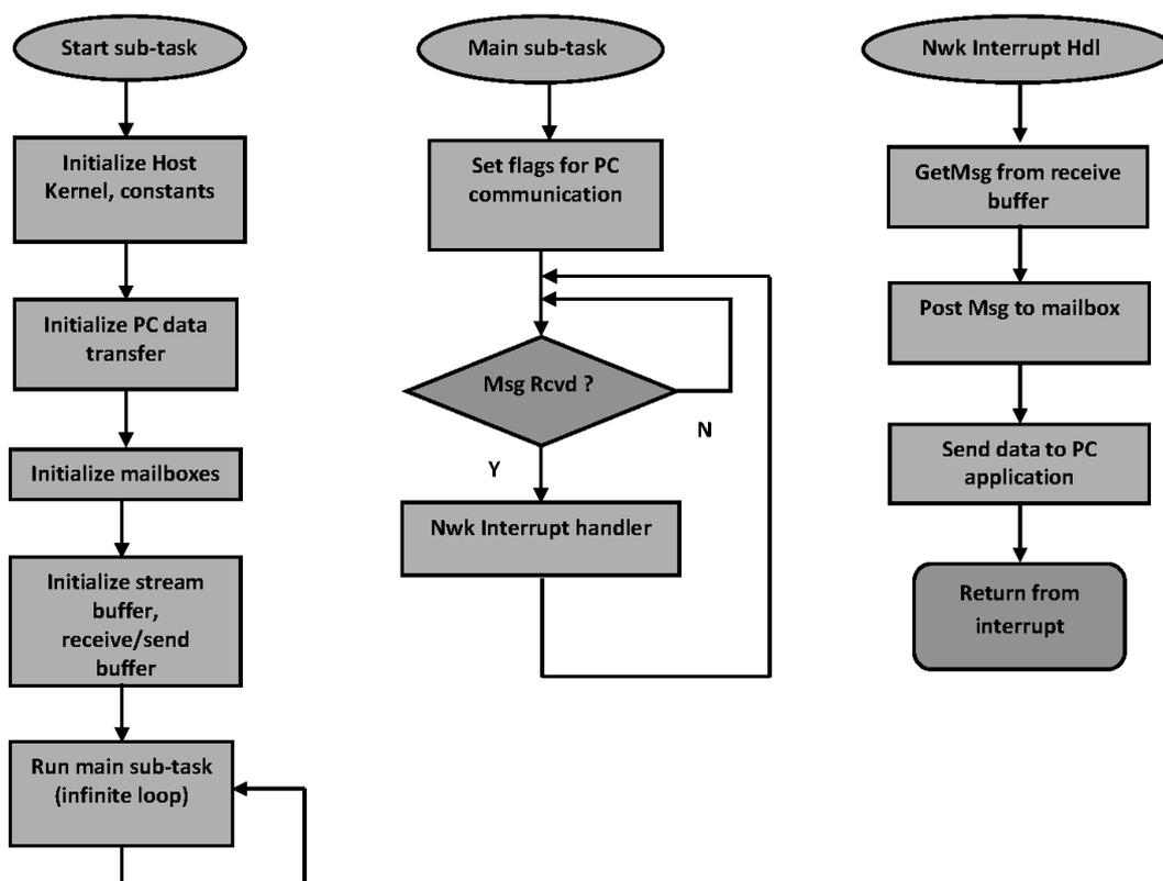
Figure 6.10: The sink sub-task model flowcharts.
