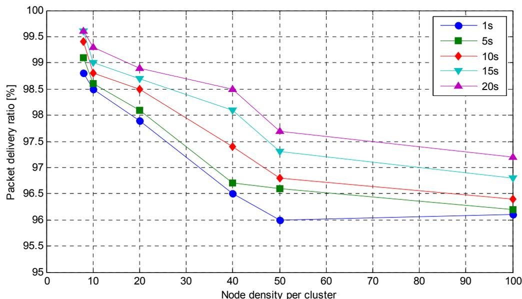
Figure 7.27: packet delivery ratio of cluster head-to-sink.
