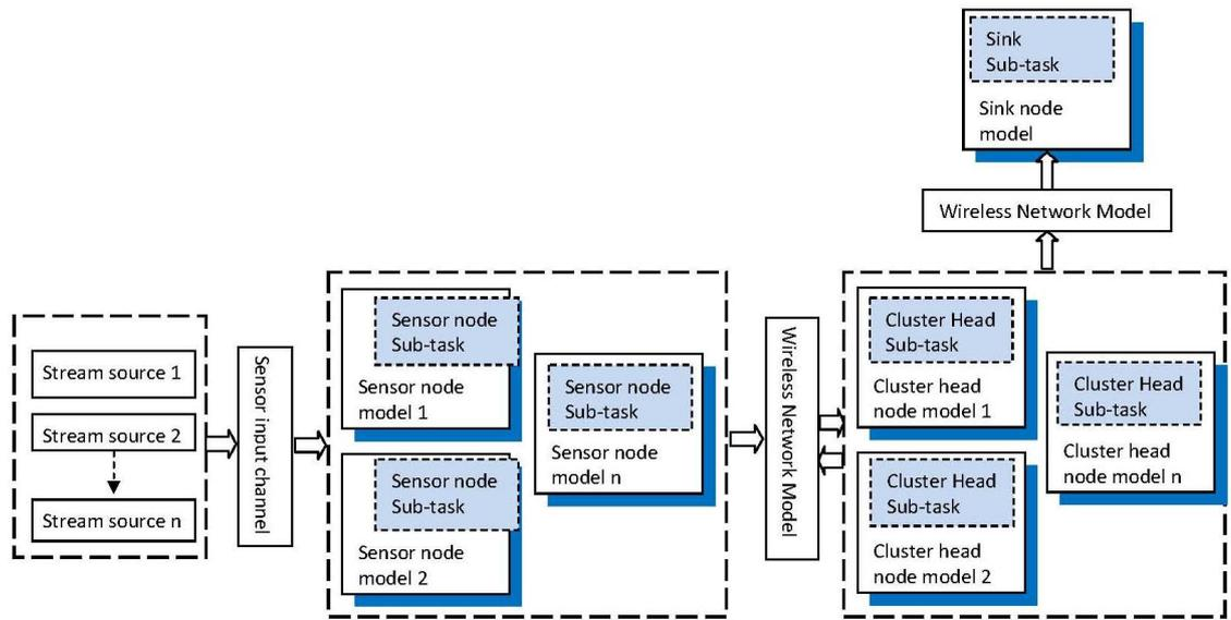
Figure 6.11: The general distributed incremental data stream mining system model.
