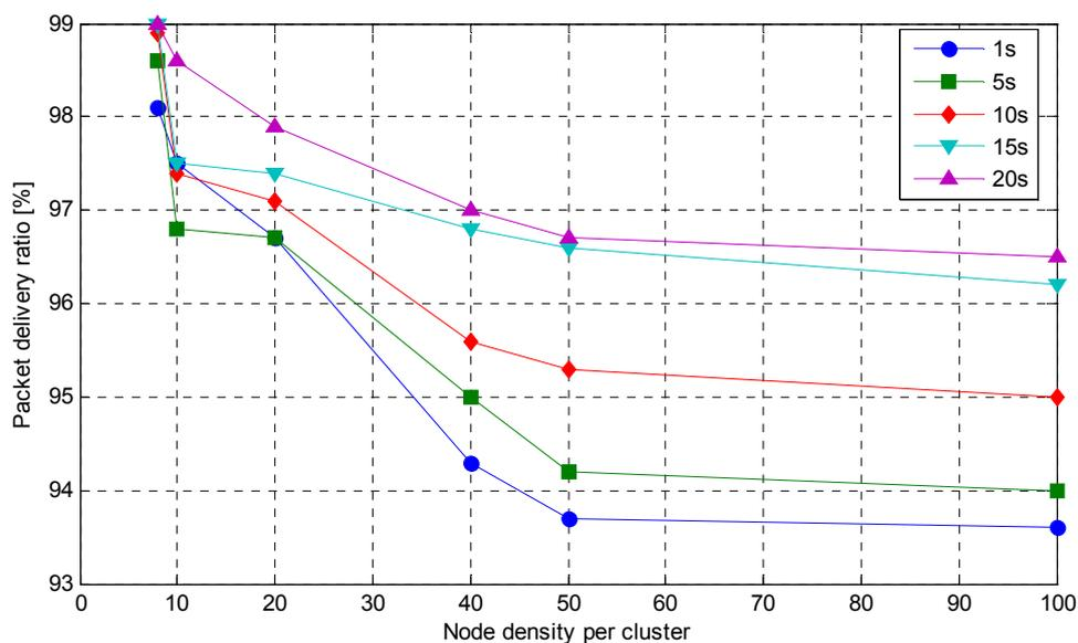
Figure 7.26: Packet delivery ratio of sensor node-to-cluster head.
