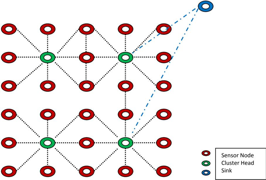
Figure 6.13: Centralized cluster-based stream clustering network.
