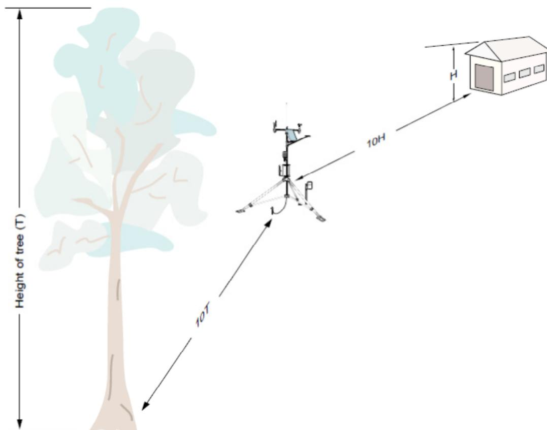
Figure 8.3: Wind speed and direction sensors siting and exposure.
