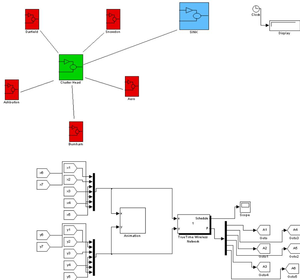
Figure 8.12: The Micro-scale FWI system model representing the Canterbury weather network.
