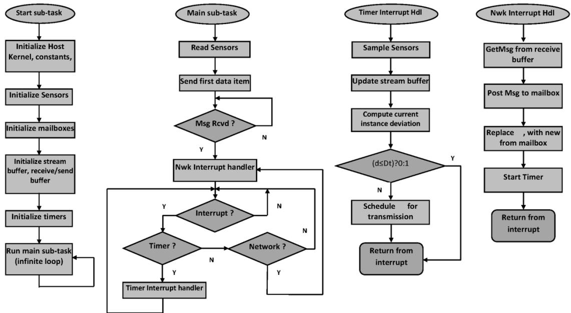
Figure 6.8: The sensor node sub-task model flowcharts.
