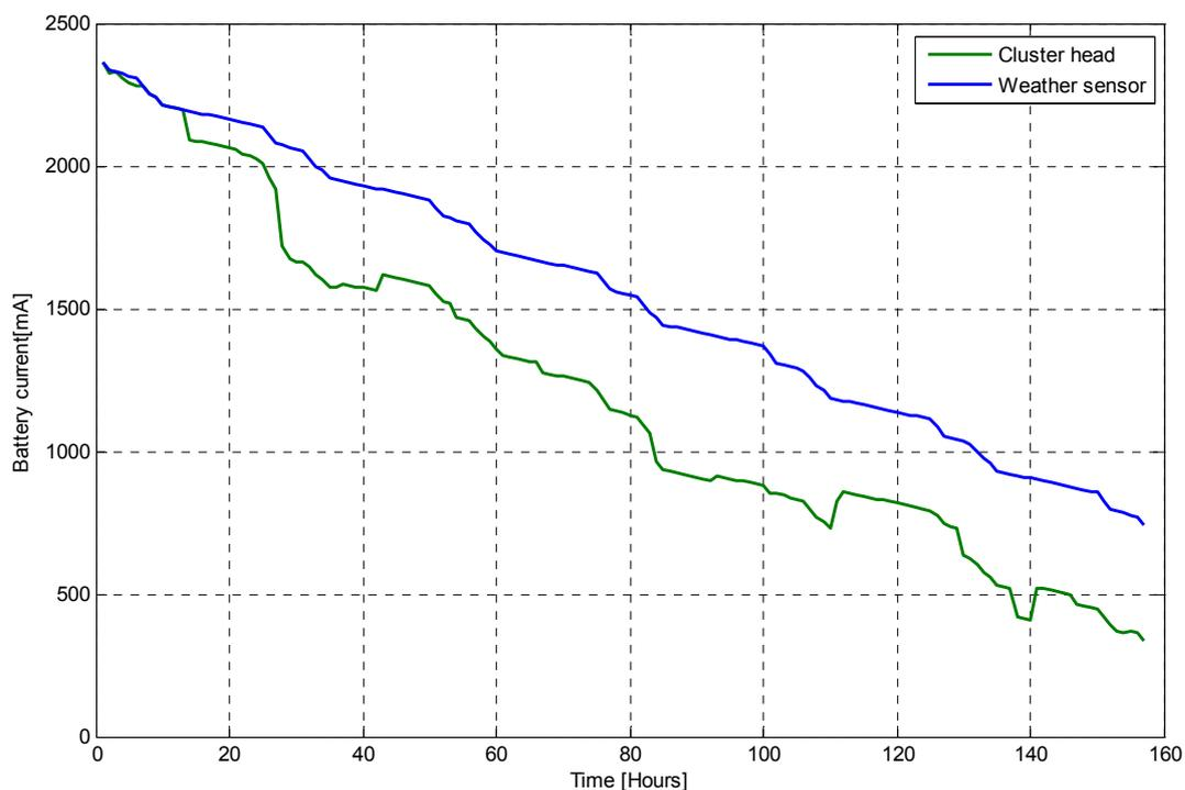
Figure 8.22: Remaining battery power of sensors and cluster heads.
