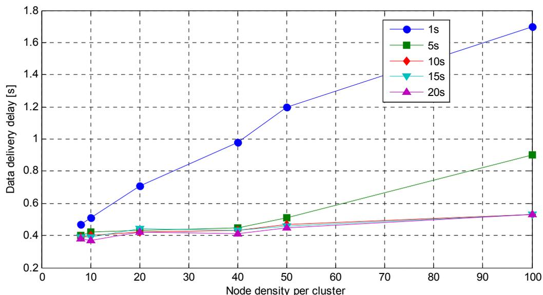
Figure 7.25: Packet delivery delay variation with cluster density.
