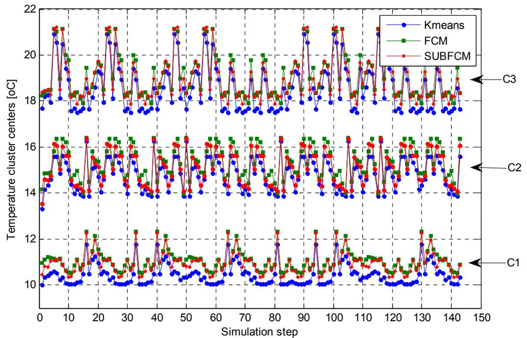
Figure 7.3: Cluster centers extracted during 144 simulation steps.
