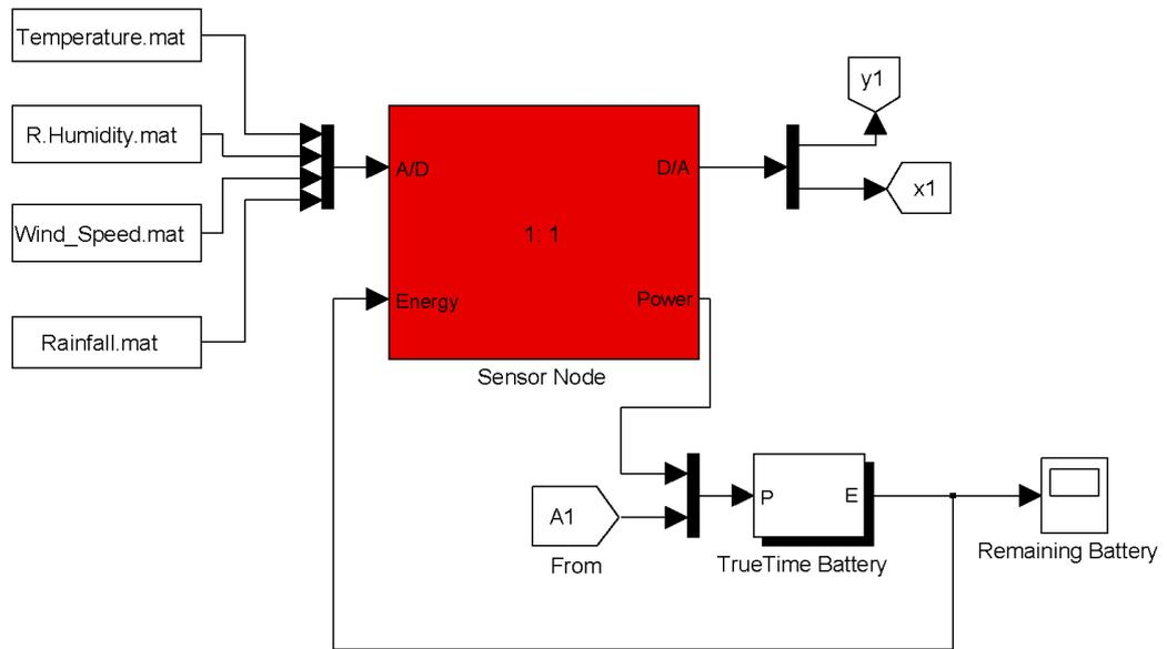
Figure 6.4: The TrueTime wireless sensor node model.
