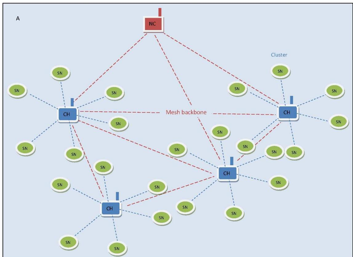
Figure 4.1: The hierarchical two-tiered WSN architecture for the distributed incremental data stream mining framework.
