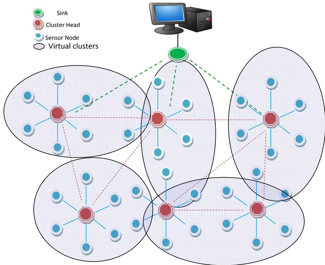
Figure 8.6: Virtual clusters of fire hazard rating or intensity mapped onto the node locations.
