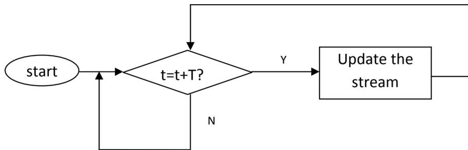
Figure 6.1: Flow chart of the sensor data stream source process.
