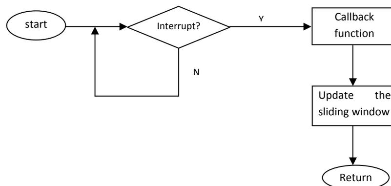
Figure 6.3: Flow chart of the cluster head data stream source process.
