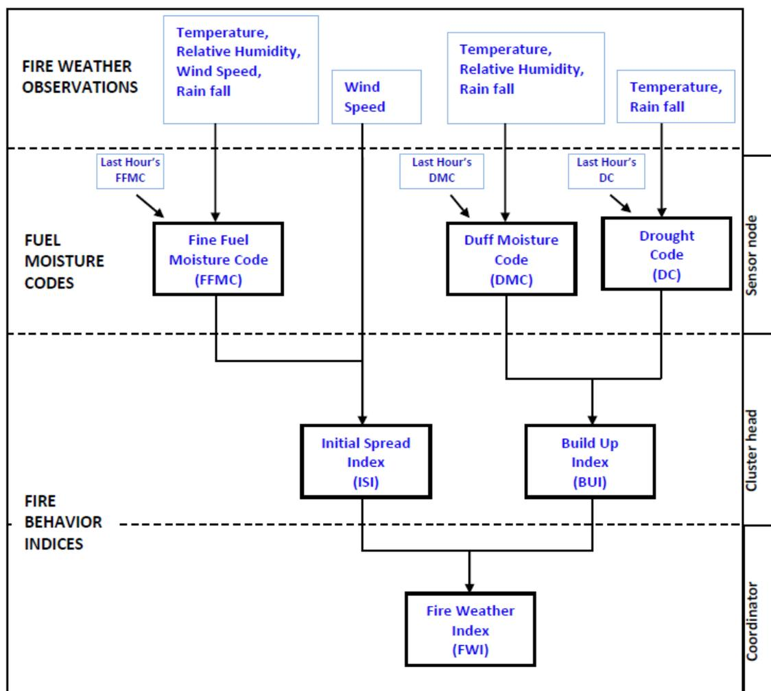
Figure 8.1: The general structure of the FWI system.
