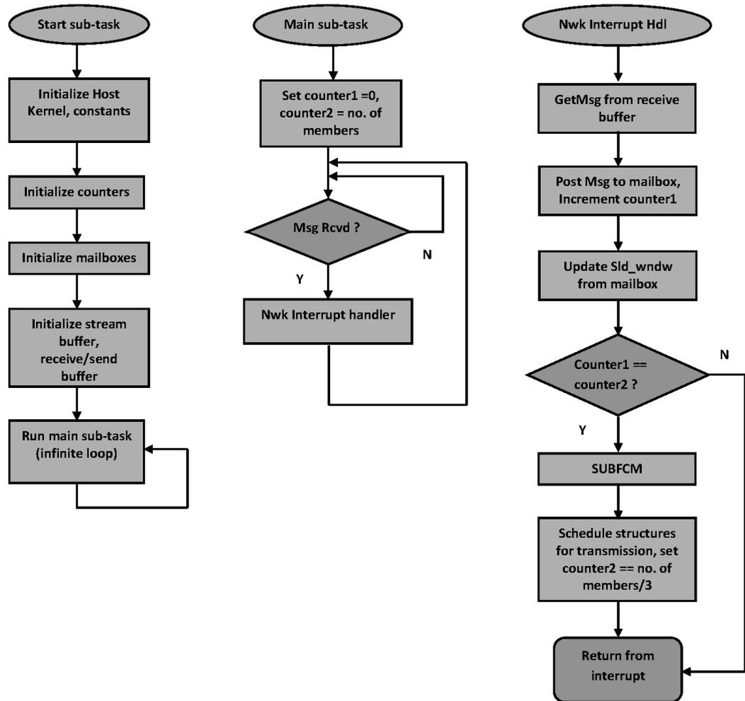
Figure 6.9: The cluster head sub-task model flowcharts.
