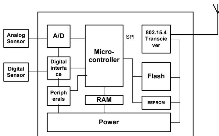
Figure 8.2: Wireless sensor node architecture.
