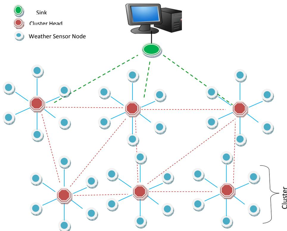
Figure 8.5: The fire weather network architecture.
