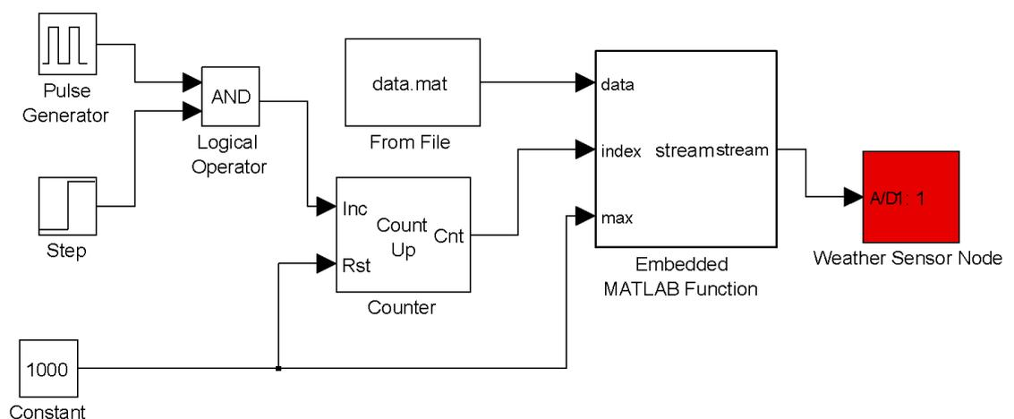
Figure 6.2: The sensor node data stream source model.
