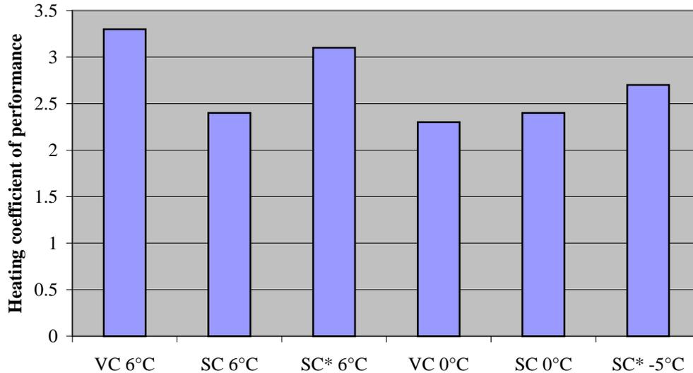
**Figure 7.** Some results from the Stirling-cycle heat-pump development programme. VC = typical vapour compression machine, SC = DH1 prior to seal development programme, SC\* = DH1 after seal development programme. The temperature stated is the outdoor temperature. The indoor temperature in all cases is 20°C.
