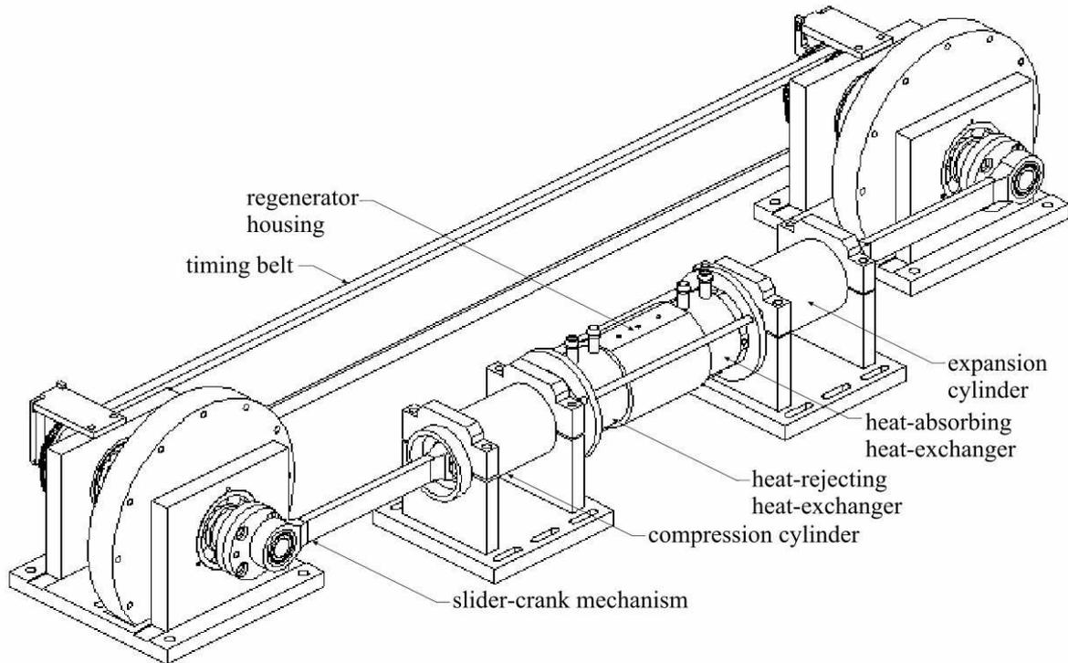
**Figure 6.** General assembly drawing of MAG1 regenerator test rig.
