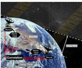
VLBI measures the arrival time delays between multiple stations utilizing radio signals from distant celestial radio sources like quasars and pulsars. In the usual geodetic VLBI analysis, clock offsets and their rates of change at each station are estimated with respect to a selected reference station.
