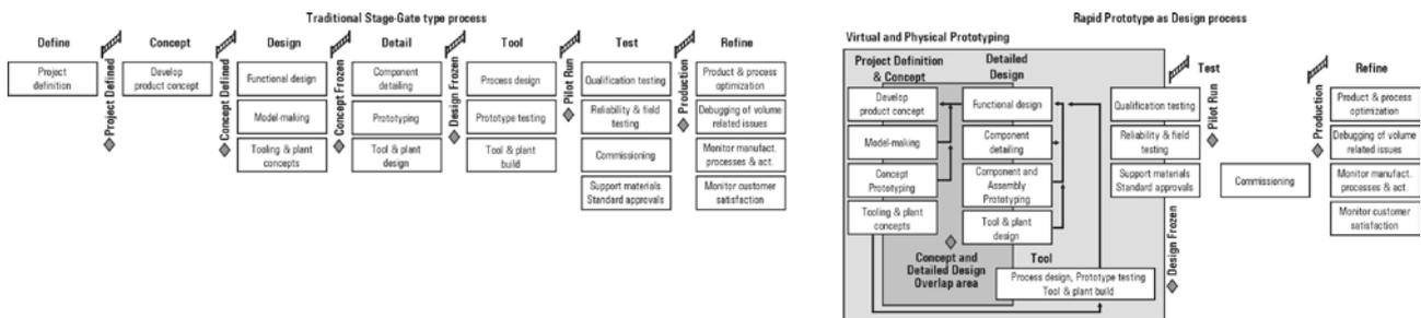
Figure 1: Comparison of Traditional and RPaD Processes
