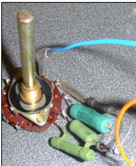
Figure 4.25 Four constant resistors soldered on four channel switch
