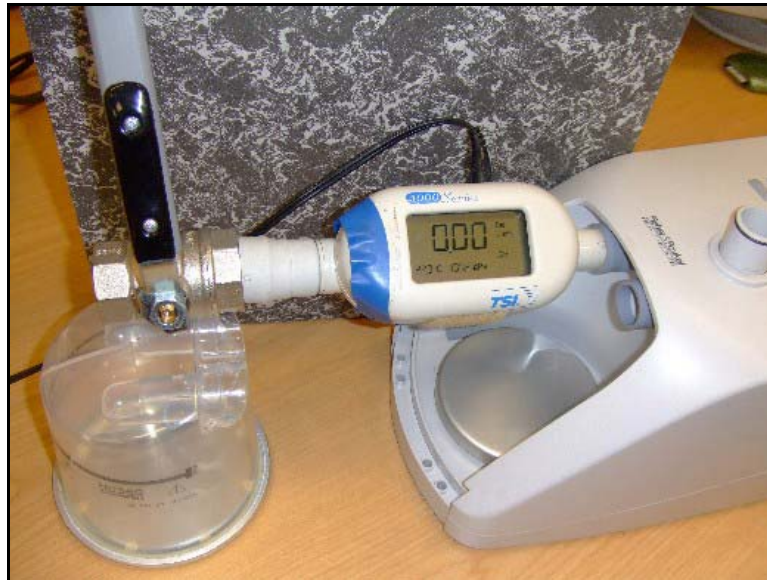
Figure 4.10 Temperature measurement of outlet of blower
