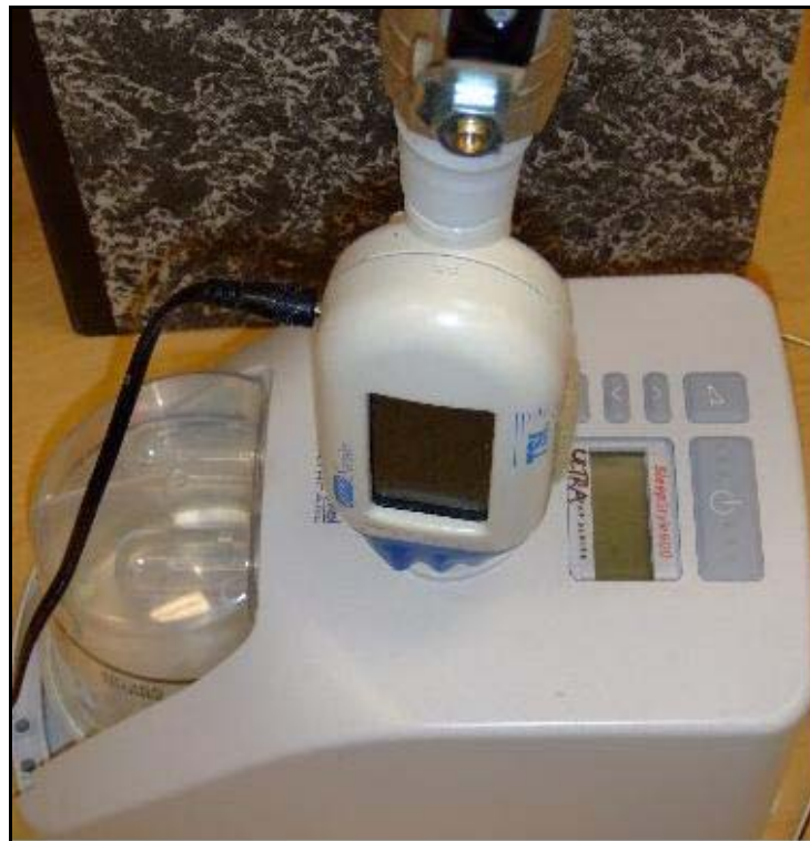
Figure 4.9 Temperature measurement of the outlet of the humidifier
