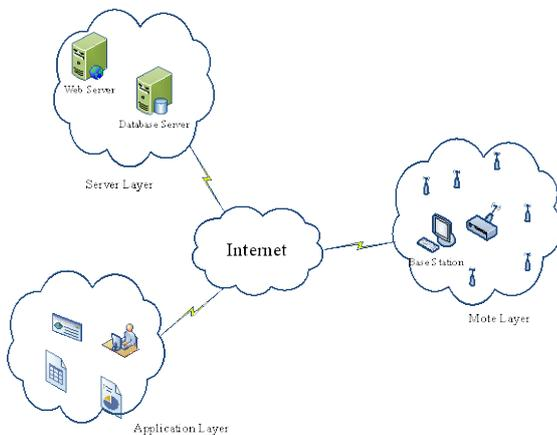
Figure 4: A schematic view of WSN architecture
