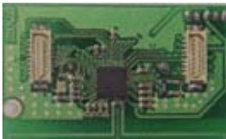
Figure 5: Wireless controller plug-in board
