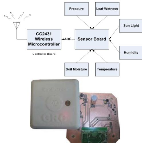
Figure 7: Router node with environmental sensors
