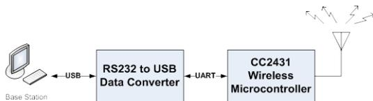
Figure 6: Base station with coordinator node
