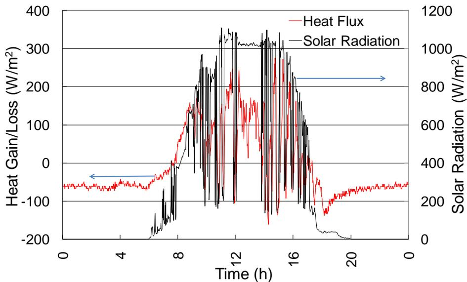
Figure 5: Heat transfer to and from the collector
