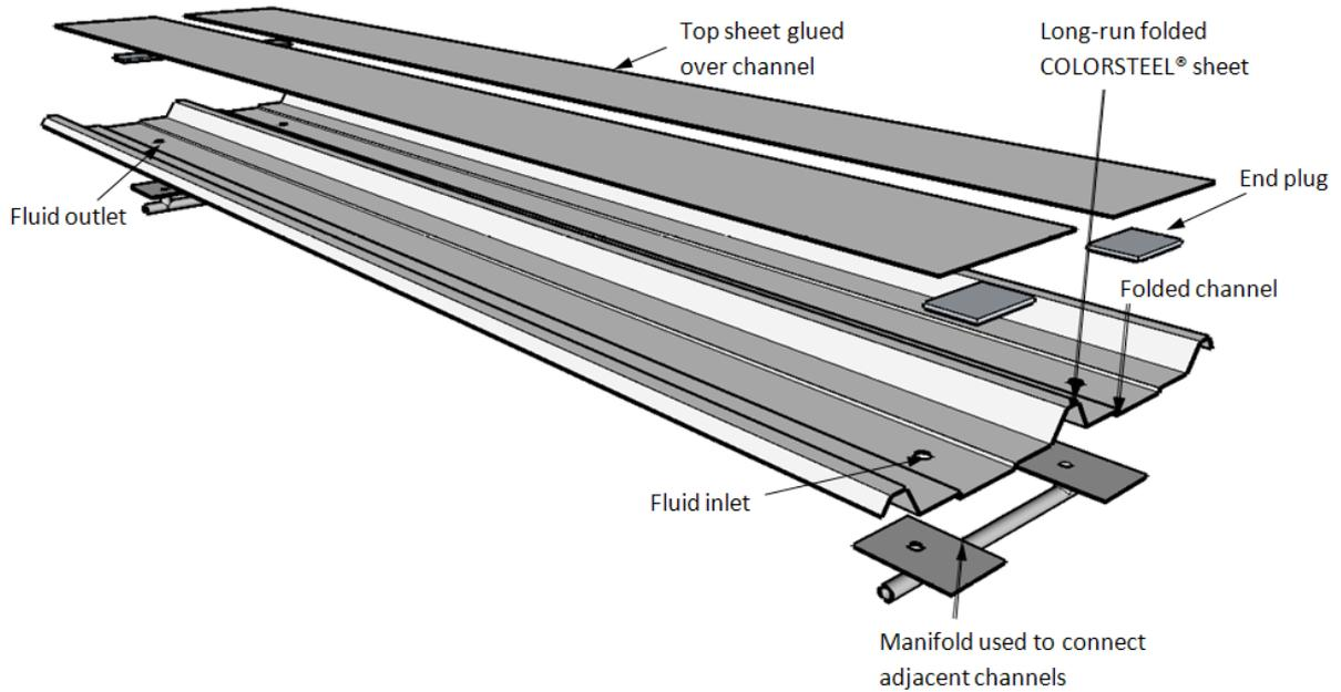
Figure 1: Building integrated collector
