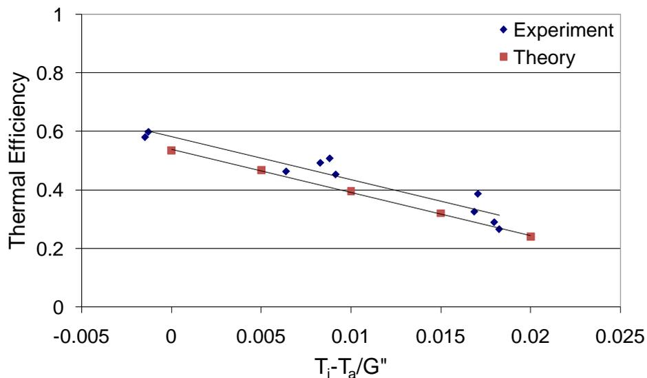
Figure 2: Thermal efficiency of unglazed solar collector
