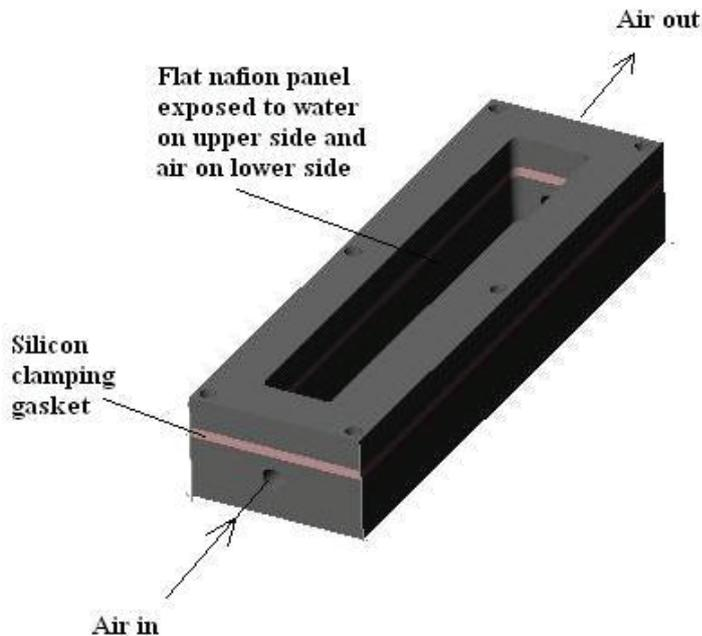
Fig. 1: Air Humidification experimental Nafion membrane holder schematic
