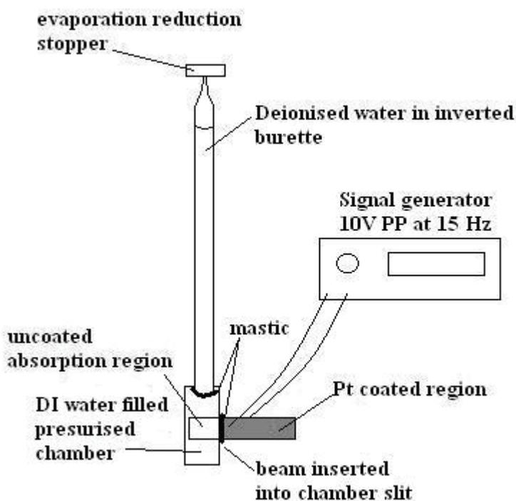
Fig. 3: End covered hydration chamber experimental schematic
