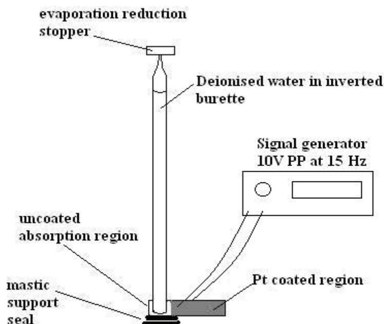
Fig. 2: Axial local surface hydration experimental set up schematic
