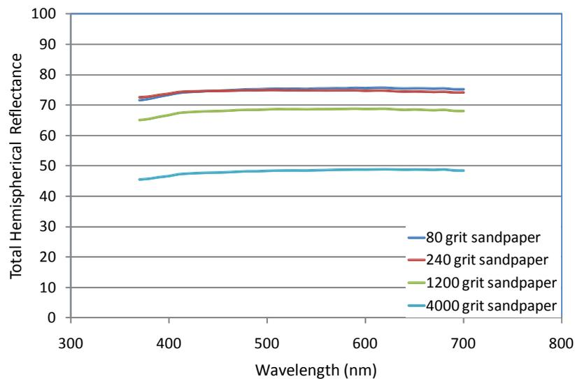
Fig. 3 Reflectance of aluminium with increasing wet/dry grit values
