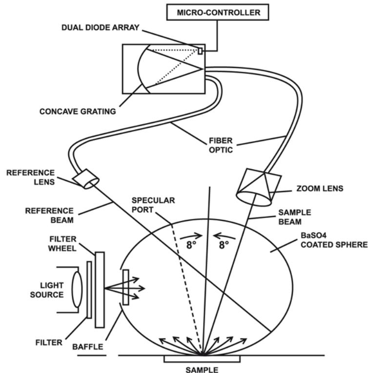
Fig. 2 Optical configuration of Datacolor 600 spectrophotometer (Datcolor, 2007)
