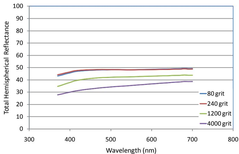
Fig. 4 Reflectance of steel with increasing wet/dry grit values
