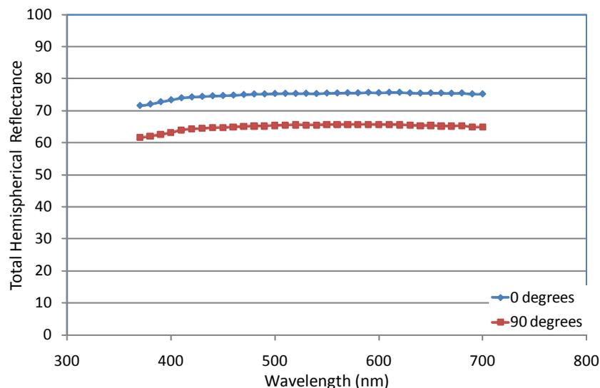
Fig. 6 Reflectance of textured aluminium samples with varying measurement orientation
