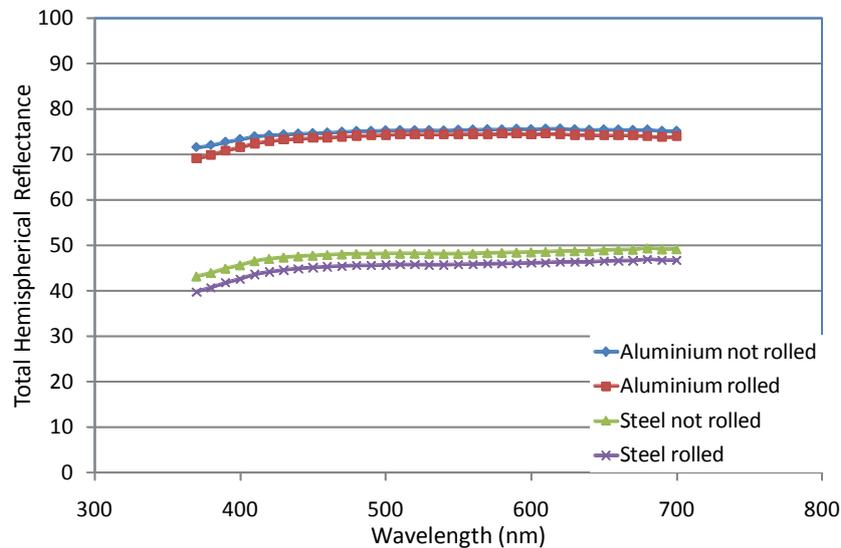
Fig. 5 Reflectance of textured samples with and without rolling
