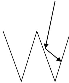
Fig. 7 Optical trapping in longitudinal surface texture features
