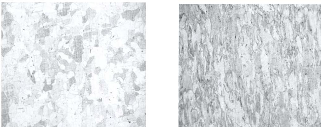
Fig. 1(a) Pre-rolled steel grain structure (b) Post-rolled elongated grain structure
