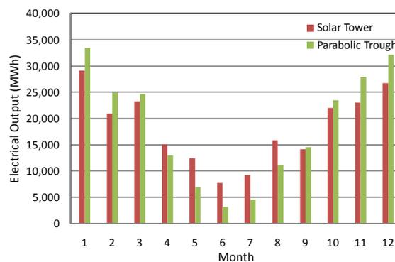
Figure 5: Output from solar power plant near Nelson
