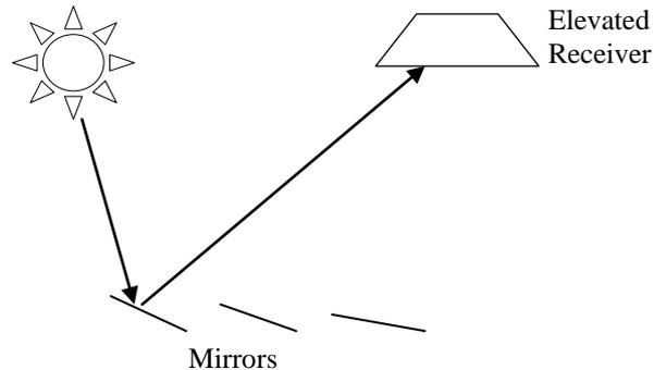
Figure 2: Schematic representation of a linear Fresnel reflector
