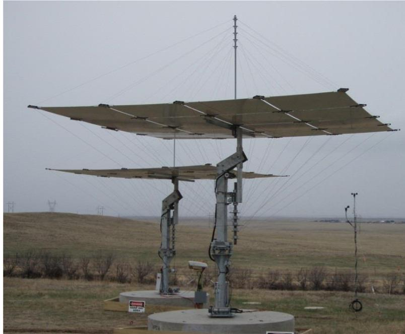
*Figure 15: Solaflect suspension heliostat*
