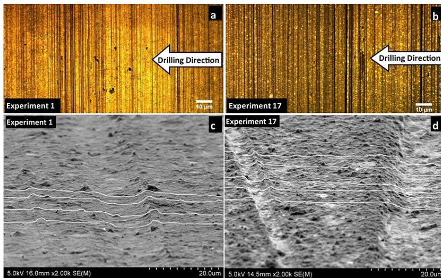
**Fig. 3: Optical micrographs of drilled surface roughness with magnification of 100X from experiments 1 & 17 (a and b) and SEM images at 2000X magnification (c and d) showing the surface roughness and the pattern of surface. Ra of 0.6 and 2.0 μm for experiment 1 and 17 respectively**
