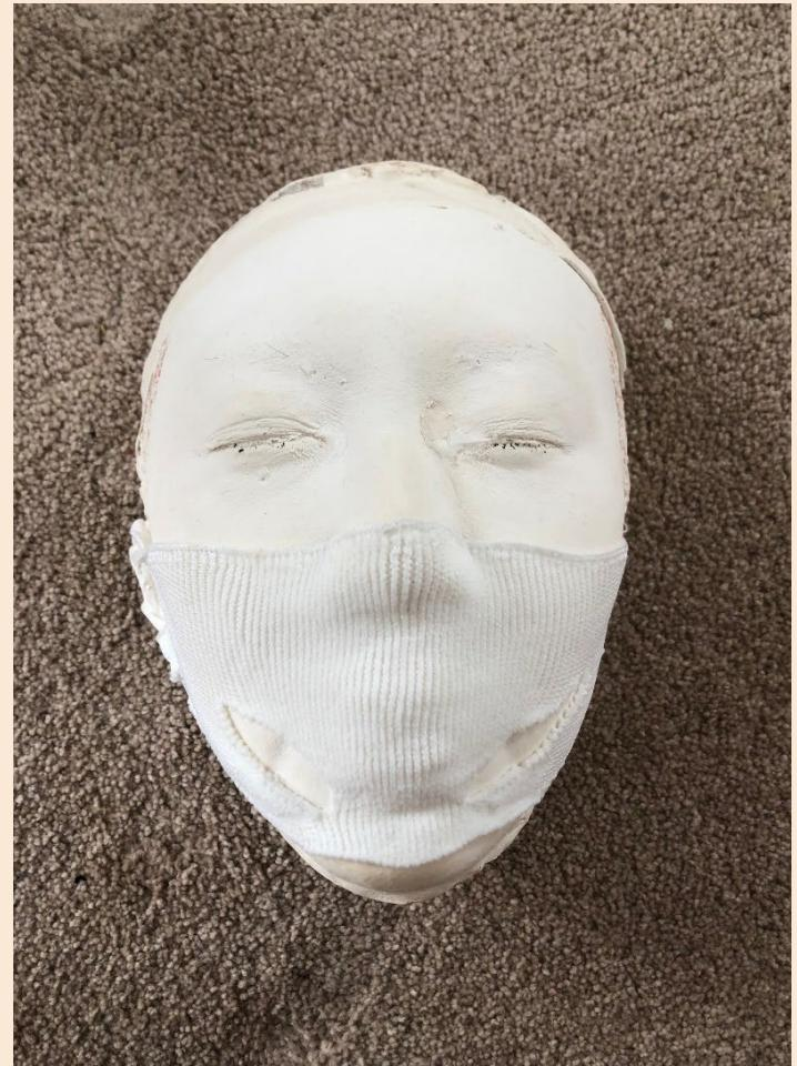
*Figure 26.* Prototype Draft IV after Heat Treatment on Face Cast.
