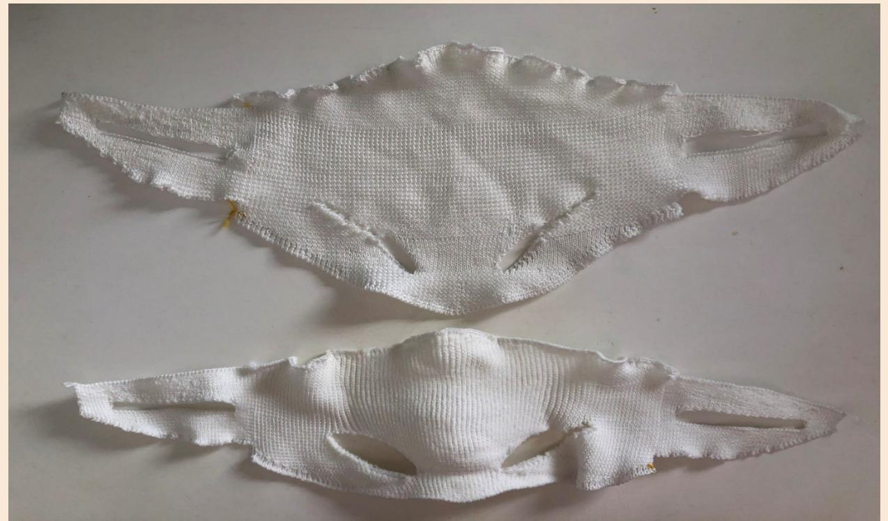
*Figure 29. Prototype Draft IV before and after Heat Treatment.*
