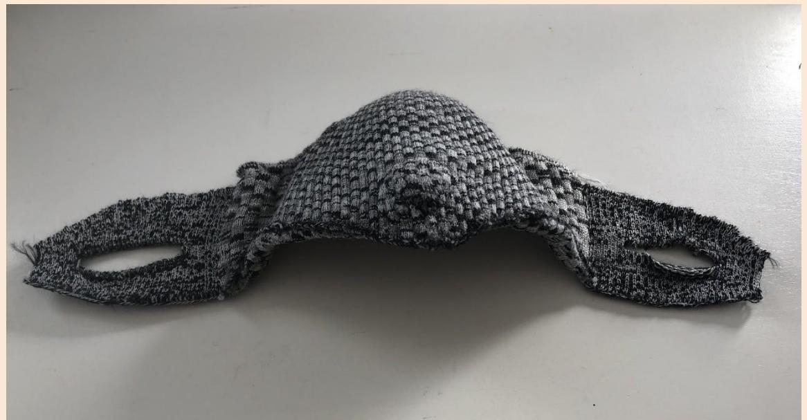
Figure 47. Popular Print Prototype Draft III After Heat treatment.
