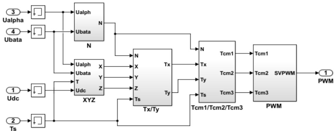
Figure 3.7: Space Vector Pulse Width Modulation (SVPWM) subsystem
