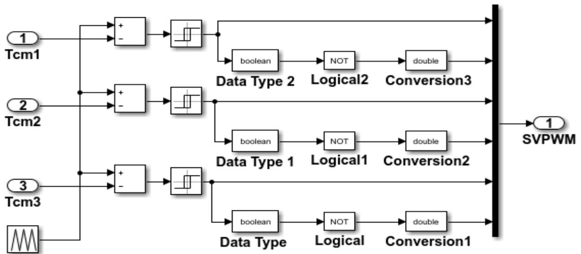
Figure 3.6: Schematics of the Pulse Width Modulation (PWM)
