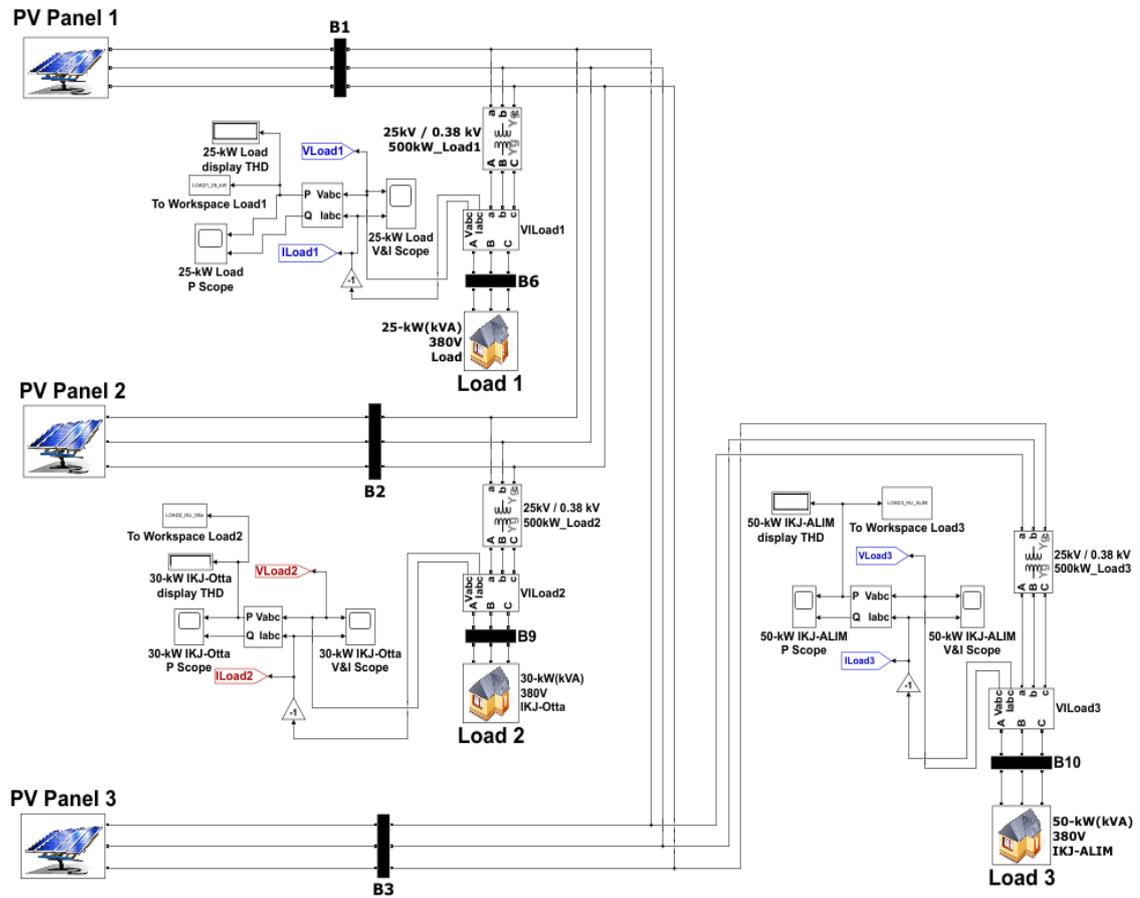
Figure 3.3: Basic concept of how a single photovoltaic system is modelled in Matlab/Simulink platform
