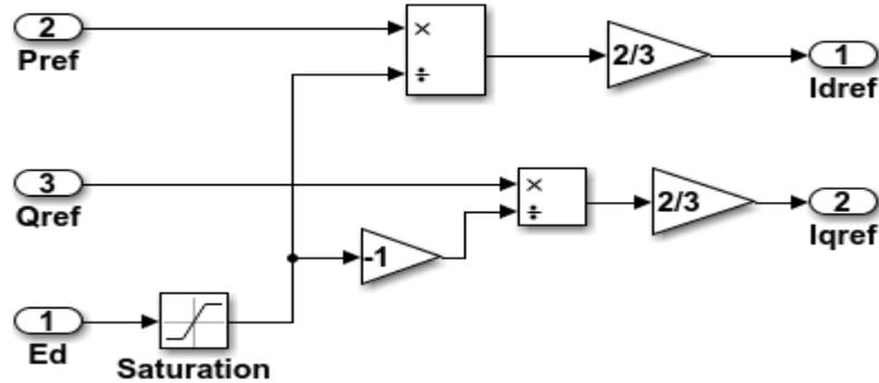
Figure 3.8: Schematics of the P-Q control subsystem
