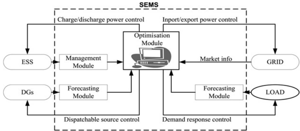
Figure 2.4: Typical illustration of SEMS inputs and outputs
