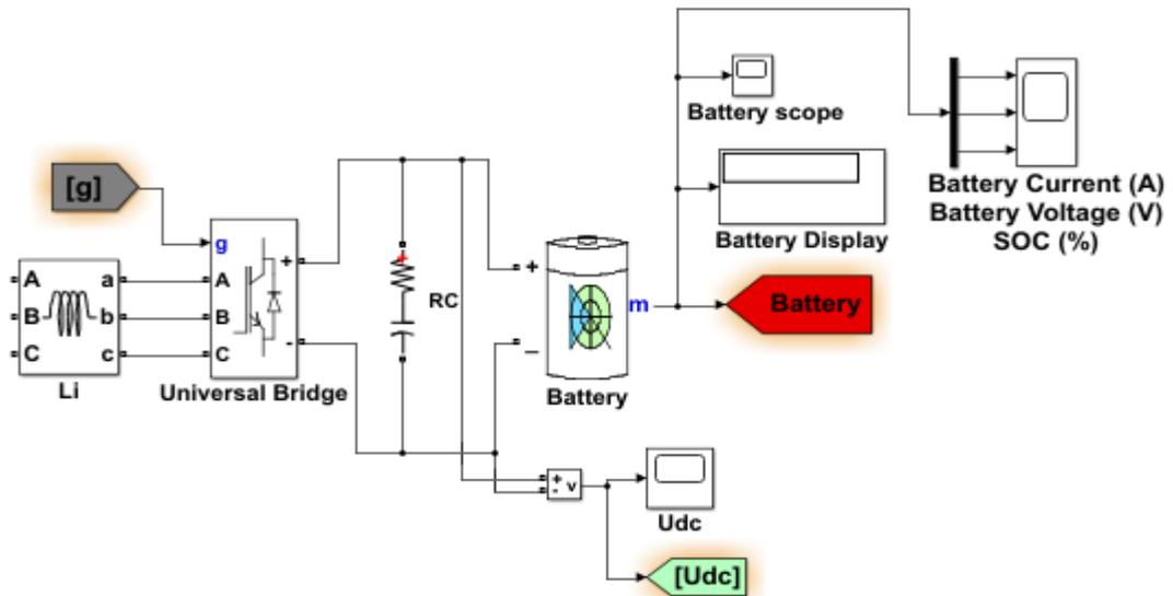
Figure 3.9: Schematics of the BESS considered for this study
