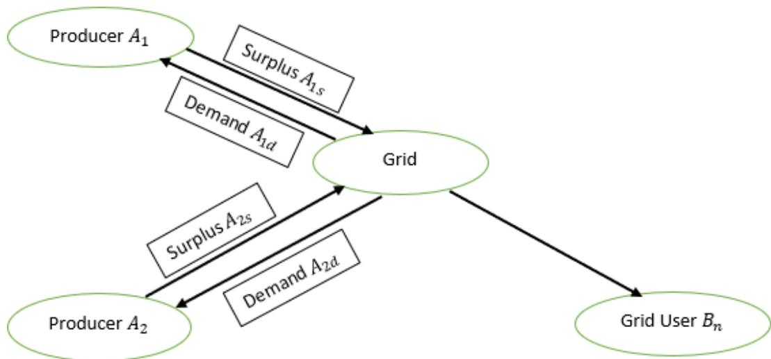
Figure 3.16: Grid serving as a storage system for energy
