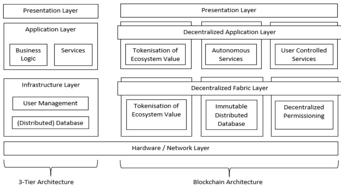
Figure 2.2: Layers of the blockchain network
