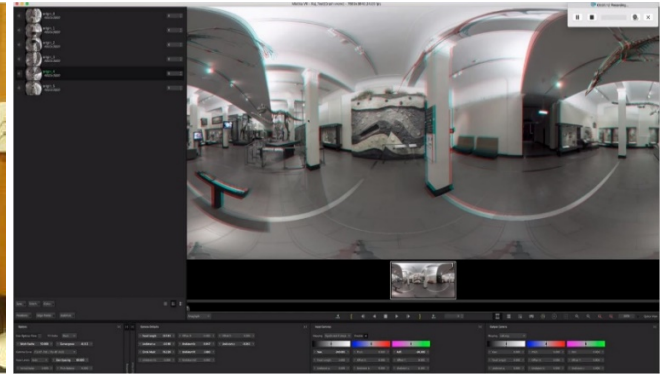
(B) Final 360 Image after stitching six images from each lens
