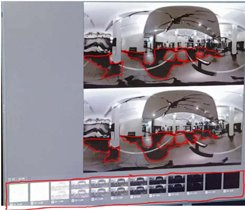
Figure 94: Resulted in black unwanted data generated during HDRI image creation by multiple lighting exposers
