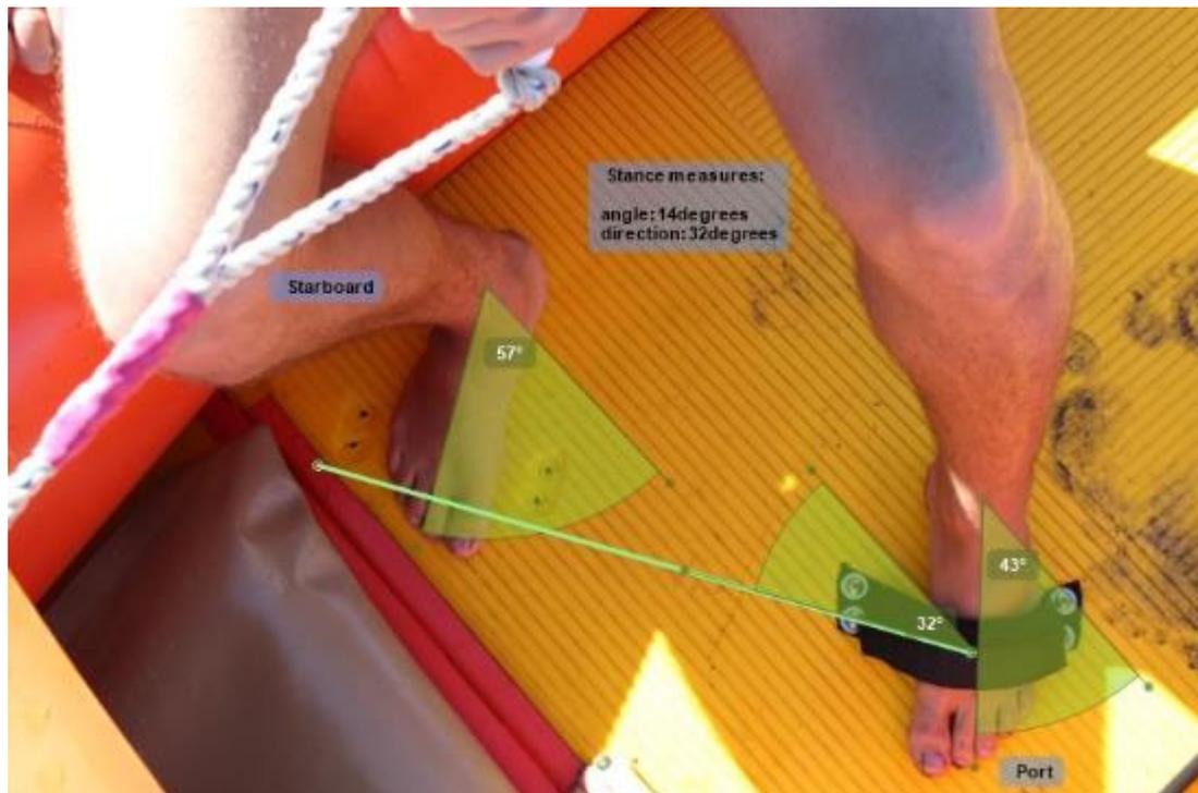
Figure 1: Stance angle and stance direction measures from photograph and Kinovea software.
