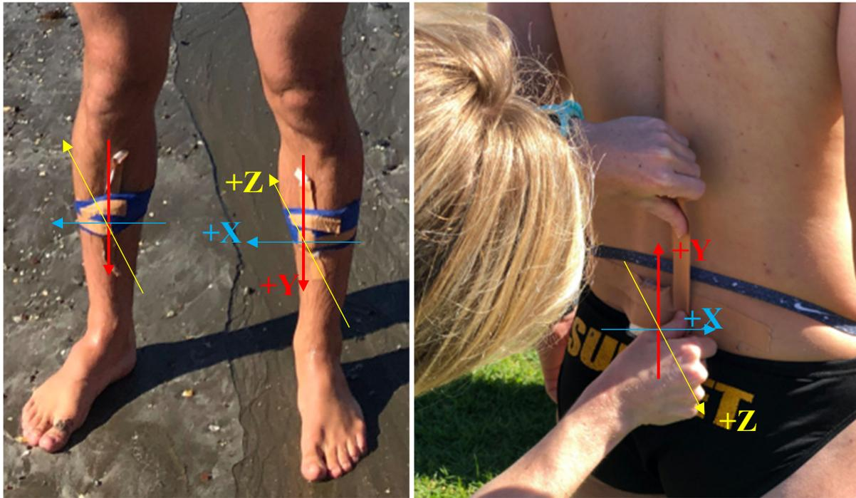
Figure 10: Inertial sensor orientations.
