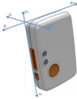
Figure 8: Shimmer3 IMU orientation.
