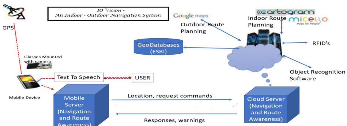
Figure 2: Components of the IO Vision System
