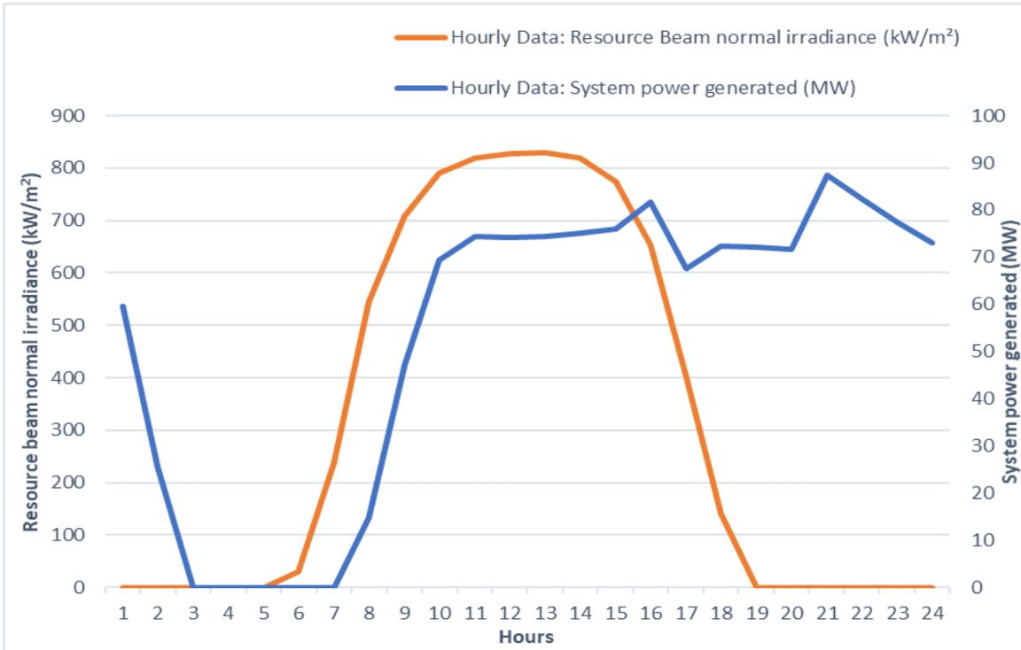
**Figure 1.**The hourly profile of the electrical energy output compared to the received DNI at the first site.
