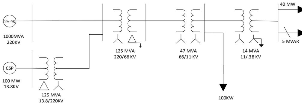
**Figure 3. Single line diagram for the proposed power system model**
