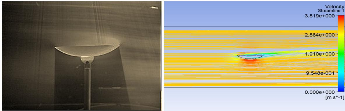
Fig 6: Flow visualization and stream lines for  $0^\circ$  tilt angle
