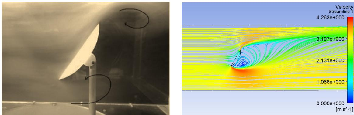
Fig 3: Flow visualization and stream lines for 60° tilt angle
