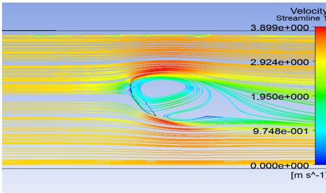
Fig 9: Flow visualization and stream lines for  $-60^\circ$  tilt angle
