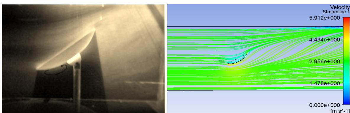
Fig 5: Flow visualization and stream lines for 30° tilt angle
