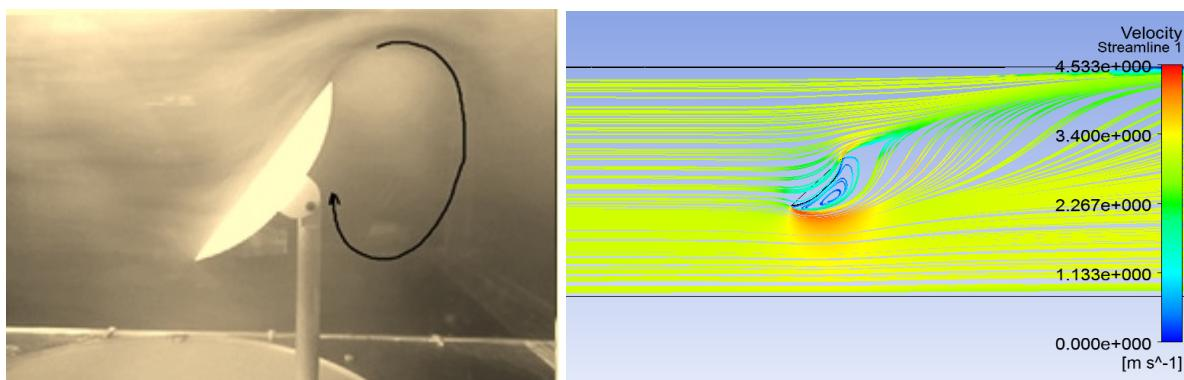
Fig 4: Flow visualization and stream lines for 45° tilt angle
