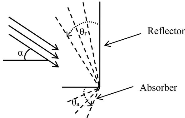
Figure 2 Angle of rotation of reflector and the absorber combination
