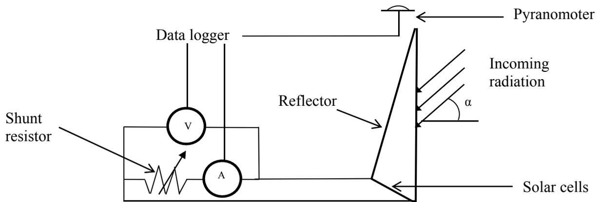
**Figure 6 Schematic diagram of the test rig**
