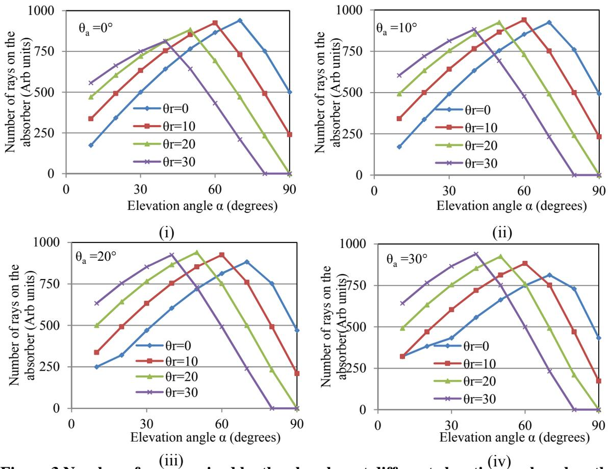
Figure 3 Number of rays received by the absorber at different elevation angles when the absorber is fixed
