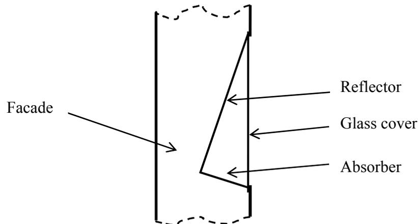
Figure 1 façade integrated concentrator
